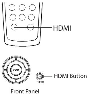
You may use the **HDMI** button on the remote control or the front panel to select the output resolution:
