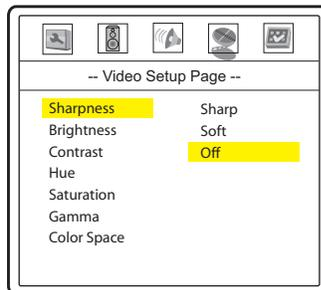
4. To select a value from the list of available settings, press the up/down **ARROW** buttons and then press the **SELECT** button to confirm.
