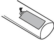
1. Remove the battery compartment cover
