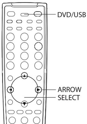
Use the **ARROW** and **SELECT** buttons to select the “REMOVABLE” item of the device selection menu, and then select the USB SLOT. The DVD player will start reading the files stored in the USB device. Please refer to page 36 for detail instructions.
