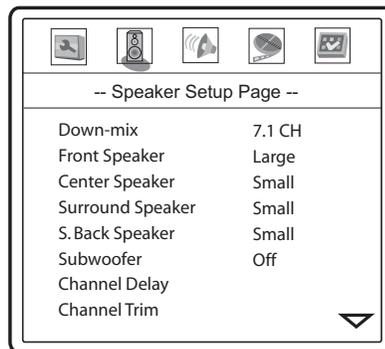
1. **Down-mix Mode:** To set the audio down-mix mode for converting multi-channel audio into two-channel output. This setting affects the analog and HDMI audio outputs. The options are:
