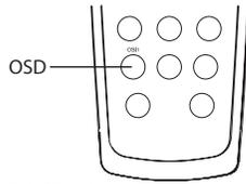
Press the **OSD** button on the remote control to show disc information and operation function hints on the TV screen.
