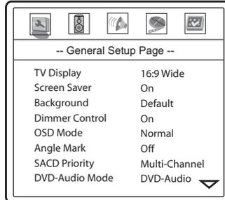
2. Press the left/right **ARROW** buttons to select the setup page. There are 5 pages: **General Setup Page**, **Speaker Setup Page**, **Audio Setup Page**, **Video Setup Page**, and **Preference Page**. Press the **SELECT** button to enter the selected setup page. The **Preference** page can only be accessed when playback is completely stopped, or when there is no disc in the player.
