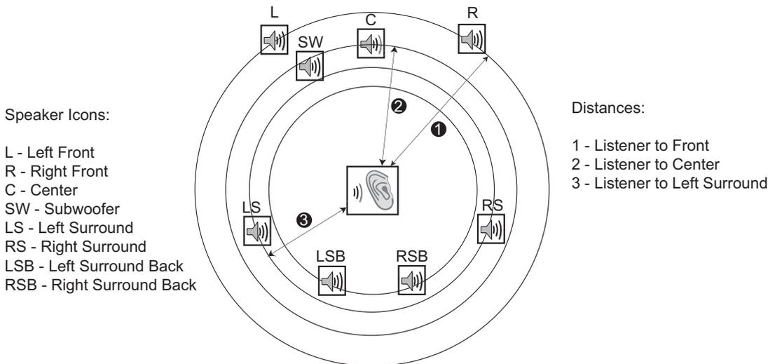
For example, in the above diagram, measure the distance (in feet) from the primary listening position to the Front Left or Front Right Speaker. Your Front Right and Left speakers should measure the same distance. If they do not, please adjust them if possible. Enter the distance of the Front Speakers (❶ in the above picture) using the left/right **ARROW** buttons.
