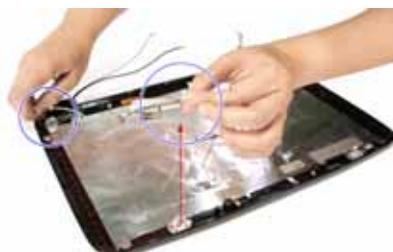
16. Detach the gasket tape holding the left antenna in place, remove the antenna bracket, then carefully remove the antenna.
