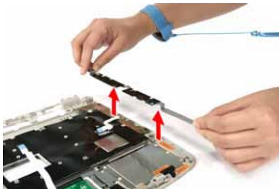
17. Remove the three screws (A) from the launch board.
