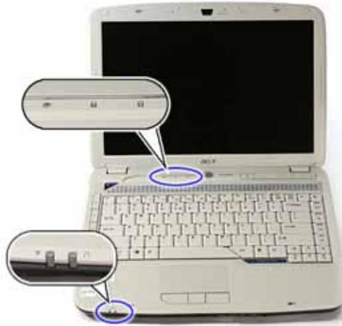
The front panel indicators are visible even when the computer cover is closed up.
