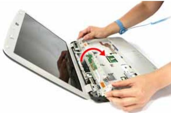
6. Using a plastic flat-blade screwdriver, pry open the connector plate then detach the media board cable from the media board.
