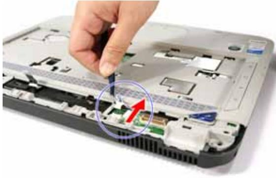
15. Detach the launch board cable from the mainboard.
