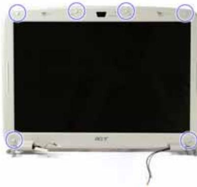
13. Remove the six screws (G) on the LCD module.
