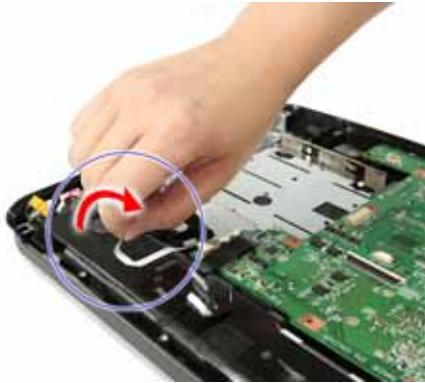
18. Detach the power board cable from the lower case.
