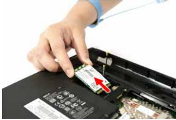
**NOTE:** When attaching the antennas back to the WLAN board, make sure the cables are routed properly.
