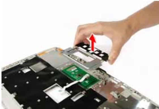
17. Carefully insert the flat screwdriver under the side of the touchpad board and gently pry up the board.
