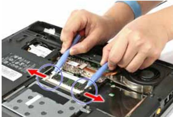
4. Remove the DIMM module.
