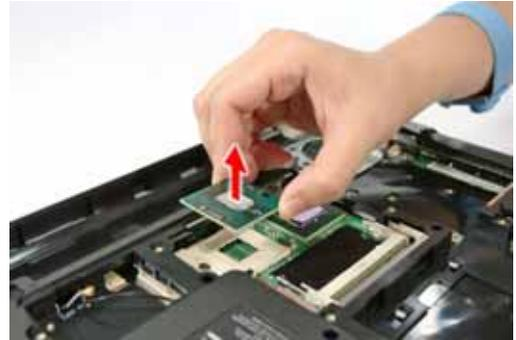
**NOTE:** When installing the CPU, make sure to install the CPU with PIN 1 at the corner as shown.
