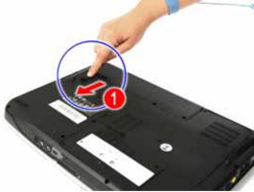
3. Slide and hold the battery release latch to the release position (2).
