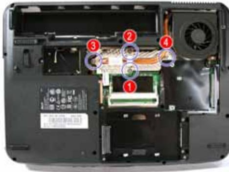
5. Remove the heatsink module.
