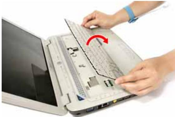
4. Disconnect the keyboard cable from the mainboard to remove the keyboard.
