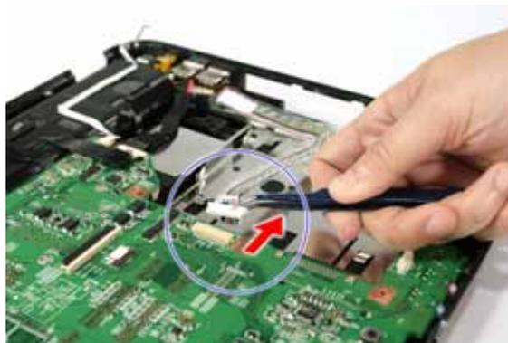
16. Pull out the AC input cable and move away from the USB board.
