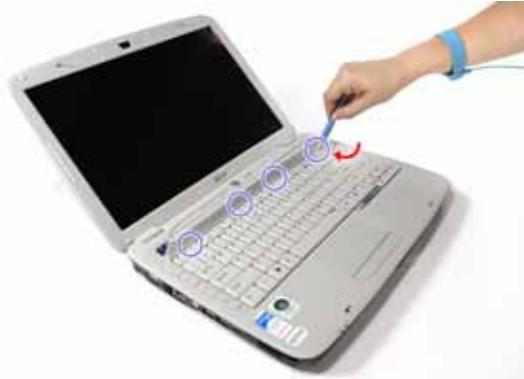
3. Carefully pry up and out the keyboard and turn it over.
