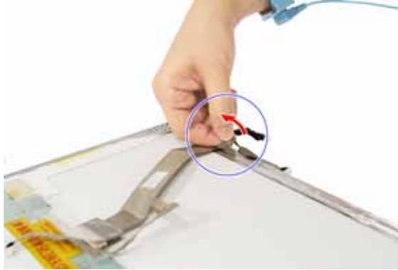
18. Detach the acetic tape securing the FPC connector.
