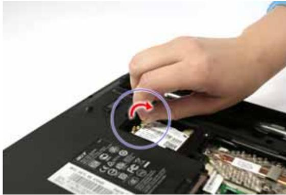
4. Disconnect the two antenna cables from the WLAN board, then move the antennas away from the board.
