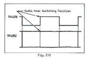
2. If the envelope has a drop out (A-portion in Fig. E11), adjust the AUDIC HEAD SW (R4281) so that the audio envelope has no drop out portion as shown in Fig. E10.
