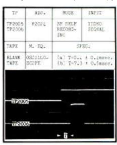
Fig. 8: Tracking fix adjustments usually require that you adjust a signal for the correct delay from the head-switching square wave.
