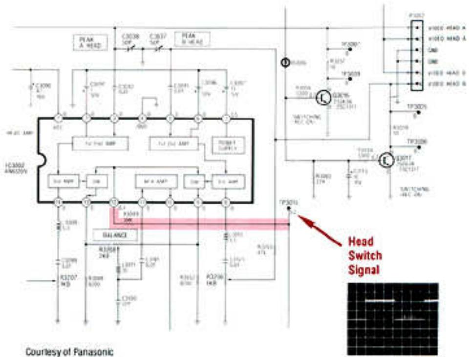
Fig. 1: The head switcher uses a 30 Hz square wave from the servo circuits to turn off the amplifiers of the head which is not contacting the tape.
