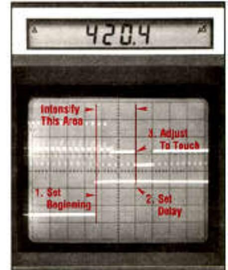
Fig. 7: Use the Delta Time function to pre-set the time needed between signals, and then adjust the circuits until the signals touch the intensified area of the waveform.
