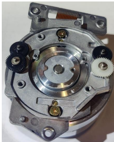
Fig 14. DD gearbox removed from video head drum, but with gears in place.
