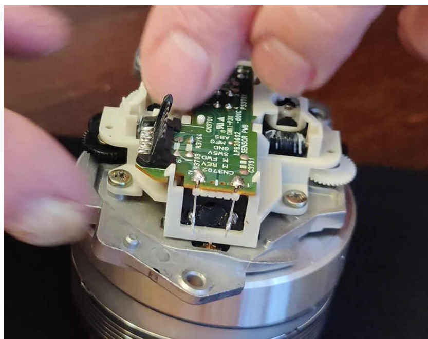
Fig 10. DD gearbox PCB removal.
