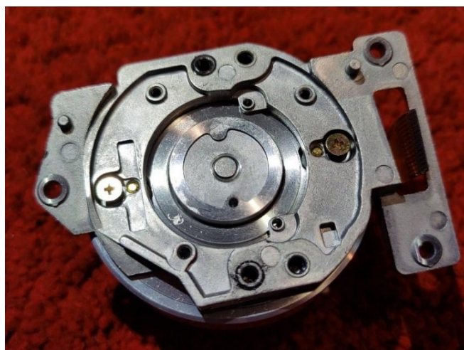
Fig. 4. Spring loaded screws, which snap the Video Drum back to neutral position.
