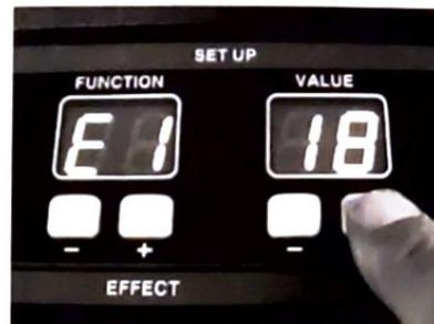
HINT: Holding down both + and - VALUE buttons together resets the display to 1.
