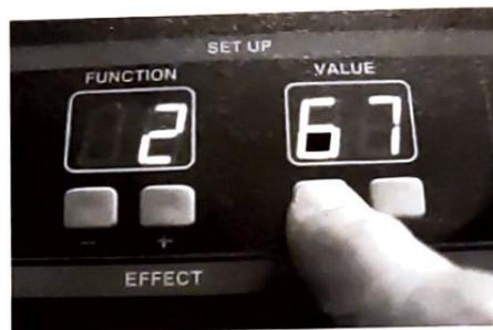
To adjust the picture using the digital processing functions, set the FUNCTION display to the function number (0-7) using the + or – buttons below the display.
