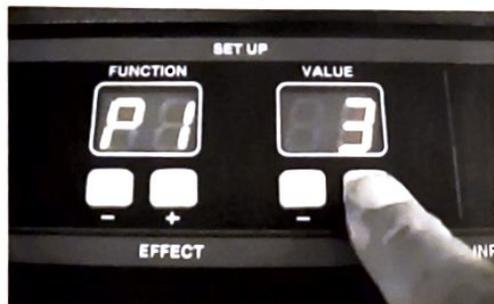
To change the PIP size, press the FUNCTION + or - buttons until the FUNCTION display shows the characters 'P1', then press the VALUE + or - buttons until the VALUE display indicates the desired size.
