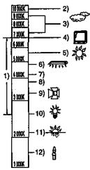
Outside of the effective range of Automatic White Balance Adjustment, the Image will become reddish or bluish. Even within the effective range of Automatic White Balance Adjustment, the Automatic White Balance Adjustment may not function properly if there is more than one light source. In this case, adjust the White Balance.
