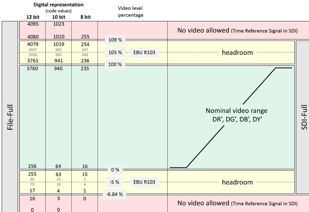
Figure 1: Typical signal levels for SDI
