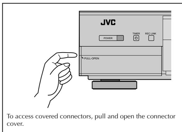
To access covered connectors, pull and open the connector cover.
