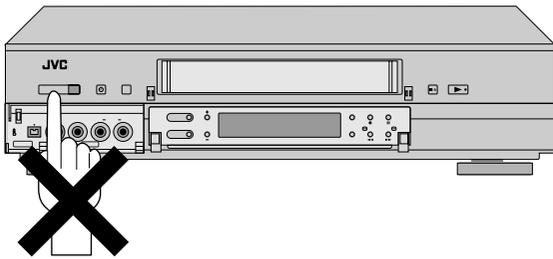
This VCR sets the clock and tuner channels automatically when AC power cord is first connected to an AC outlet. The antenna cable must be connected for the Plug & Play setting.
