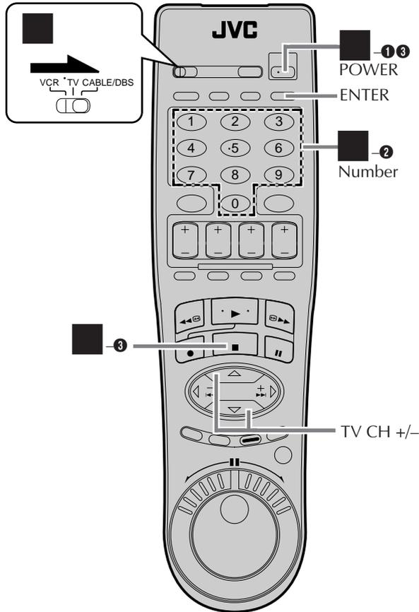
This Remote can control some functions of the DBS (Direct Broadcast Satellite) receivers listed below.
