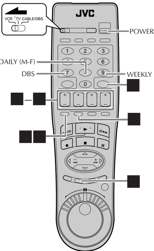
You can directly program the VCR's timer to record up to 8 broadcasts, as far as a year in advance. Remember, the clock must be set before you can program the timer (→ pg. 10).
