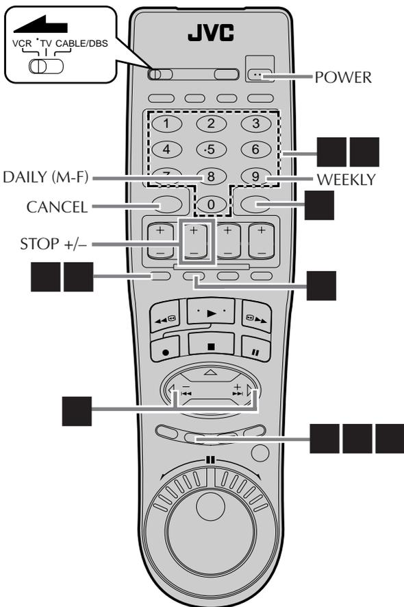
Timer recording allows you to program the VCR to automatically record a broadcast at some future time. Up to 8 timer recording programs can be made using VCR Plus+ timer programming or Express timer programming method (see pg. 38) as far as a year in advance.
