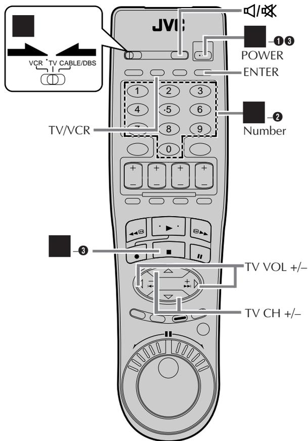
This Remote can control some functions of remote controllable TVs listed below. Without setting, you can control a JVC TV.
