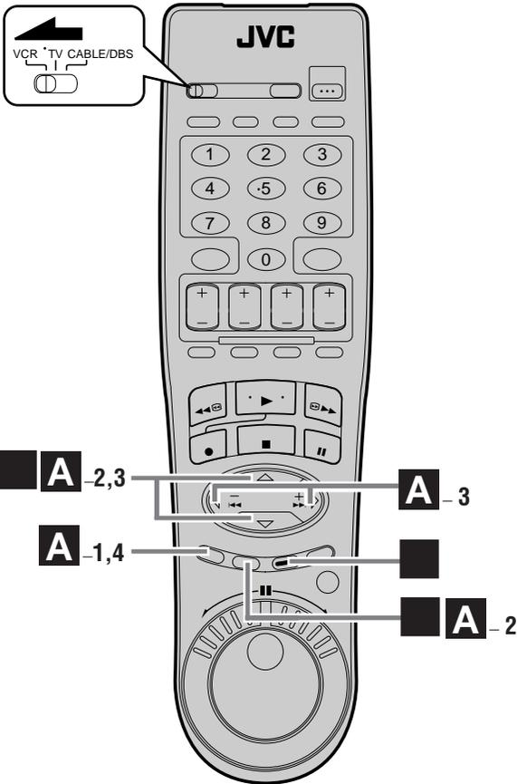
This function is useful when you want to quickly find out what programs you have recorded on a tape using this VCR. This function allows you to select a program to watch, and then automatically searches for the beginning of the program.
