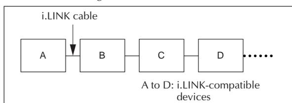
Any two devices in the daisy chain can exchange data bi-directionally, even if there are other devices connected between them.
