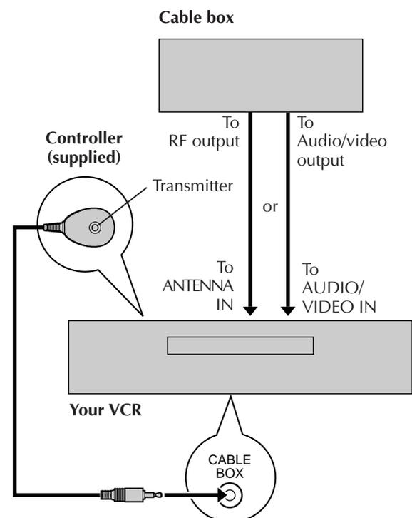
The following procedure is required if you receive your TV channels through a cable box (descrambler). The Controller allows the VCR to automatically switch the cable box channel during timer recording. The Controller is effective for recording broadcasts that have been programmed using VCR Plus+ (☞ pg. 34) or Express timer programming (☞ pg. 38).
