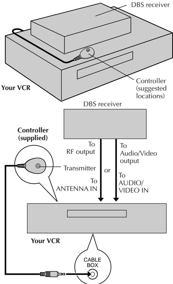
The following procedure is required if you receive satellite channels through a DBS (Direct Broadcast Satellite) receiver. The Controller allows the VCR to automatically switch the DBS receiver's channels during timer recording.
