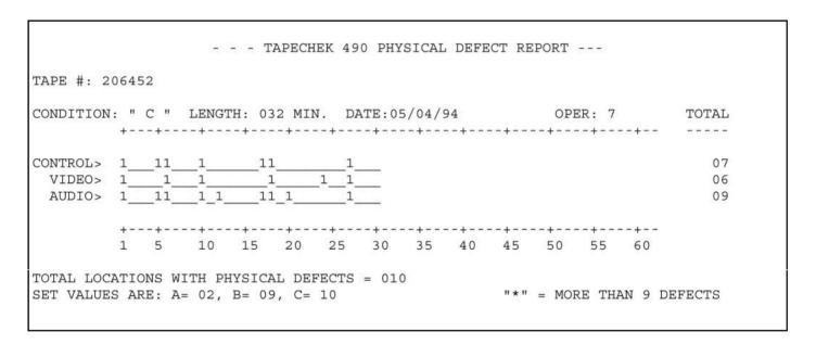
As you can see, the report prints out the inspection data as well as a graphic representation of the locations of defects found and the total tape length (in minutes of playing time, SP speed).
