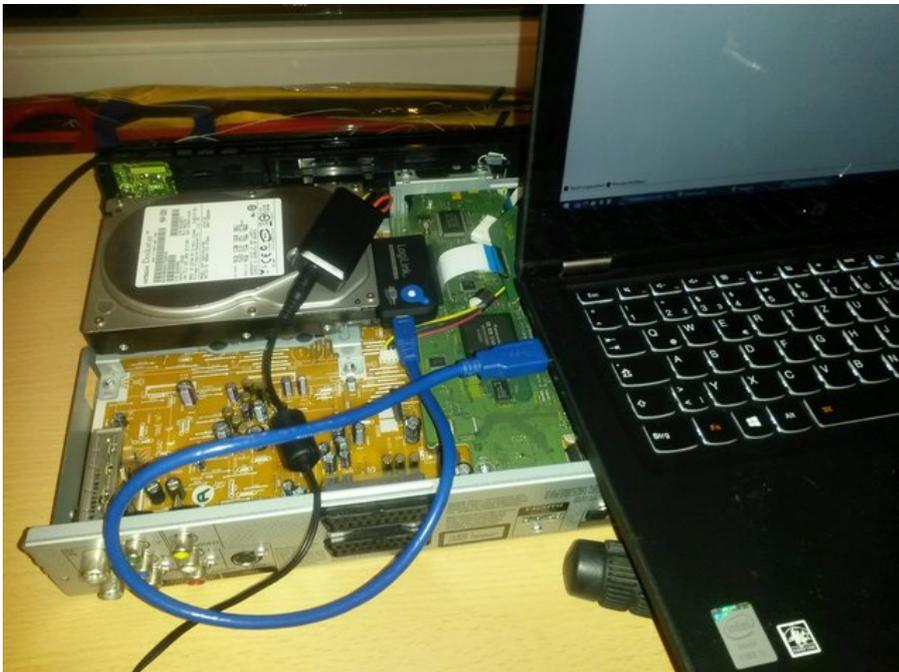
Now it should be checked whether the drive has been correctly recognized by the PC (in the case of direct connection, first in the BIOS / UEFI - otherwise in the Windows Device Manager).
