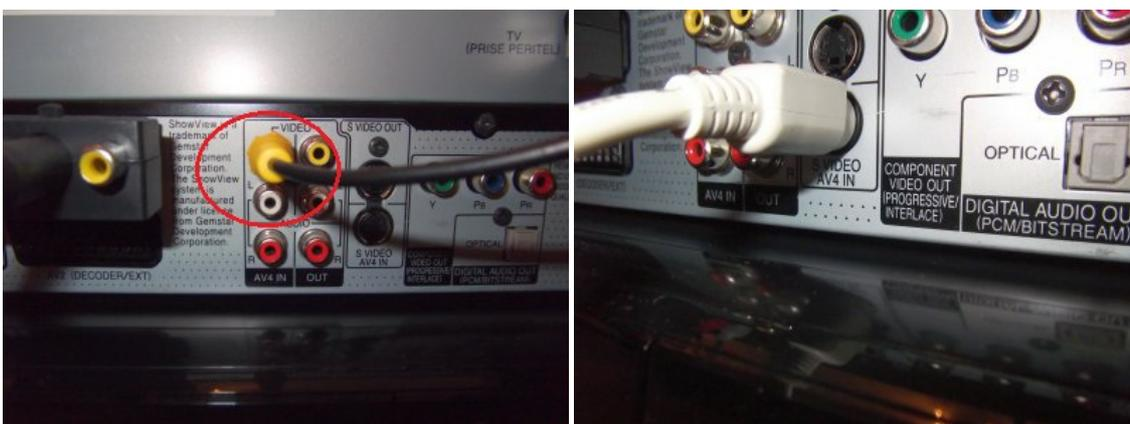
The connection to the DMR-ES10 can also be made via Scart to AV2 (although it only depends on the image signal), if the source device has again separate audio outputs, which can then be connected directly to the terminal. In this case, the AV2 input in the setup menu of the DMR-ES10 must be configured for the correct input signal (CVBS or S-video). This is similar to the newer models (see above). The direct connection is easier and less error-prone.
