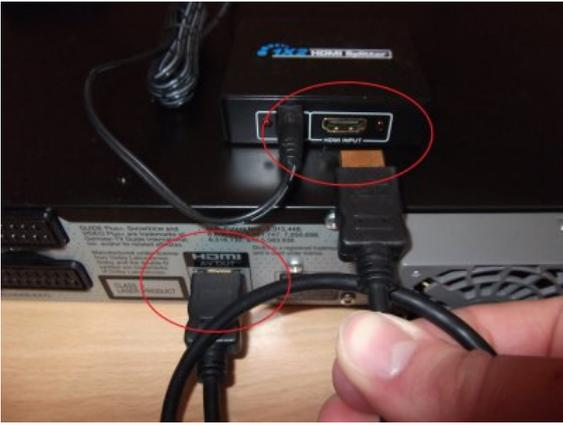
2. Any output of the splitter will be connected to the HDMI input of the Intensity card
