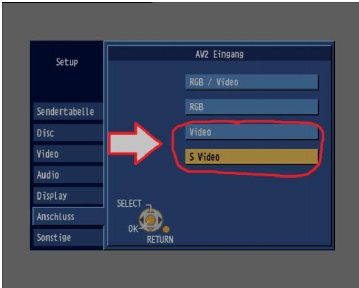
If a pure VHS recorder is connected via scart, "Video" must always be selected.
