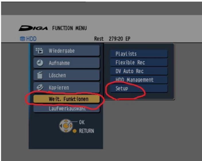
First, the main menu must be accessed via the "FUNCTION MENU" button on the remote control, and then via "Far. Funktionen -> Setup" the Setup Configuration menu will be invoked. The navigation and selection is done with the directional pad, the OK button and RETURN.
