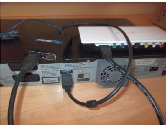
This cabling is already sufficient for operation. To avoid any difficulty in getting the Intensity card into operation for the first time and configuring the DVD recorder, as well as for general control over the ongoing dubbing, it may be advisable to connect another TV / monitor to the DVD recorder that controls the output of the DVD Plays back.
