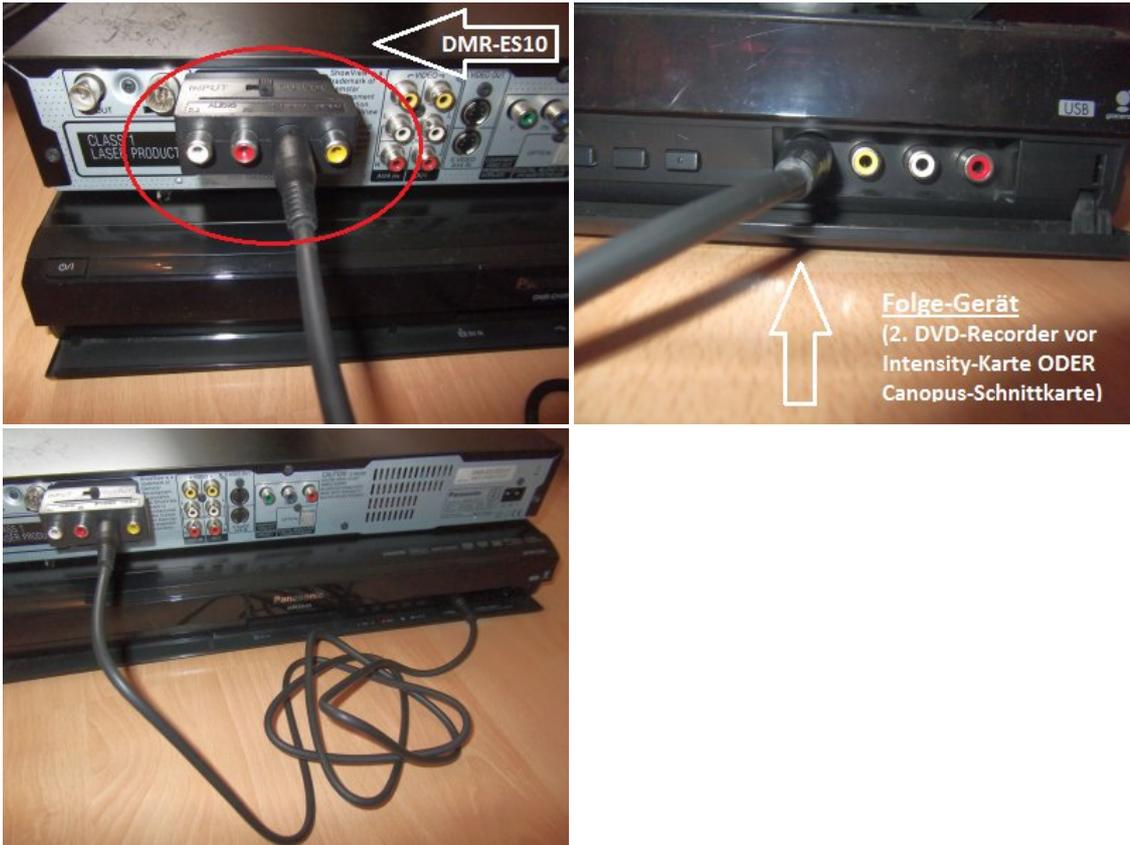
Next, only the VIDEO signal of the tape device is connected to any input of the DMR-ES10. Since the DMR-ES10 (and also DMR-EH52 / -EH50 / -EH60) has rear separate inputs for CVBS or S-video (AV4), you can use this (or the front inputs (AV3)). Depending on whether you connect a VHS device via CVBS or an S-VHS device via S-Video, the connection looks like this:
