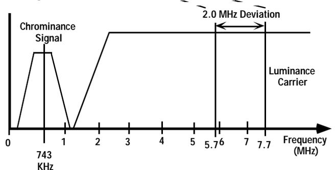
*Fig. 5: U-Matic SP raises the luminance frequency to improve resolution from the existing format.*
