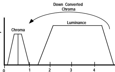
Fig 1: The frequency of the chroma signal is down-converted in the VCR "color under" format.
