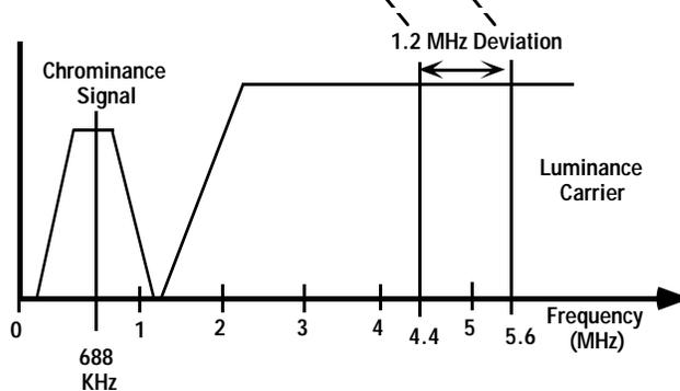
Fig. 4: The Super Beta format raises the luminance frequency to improve resolution from the existing format.
