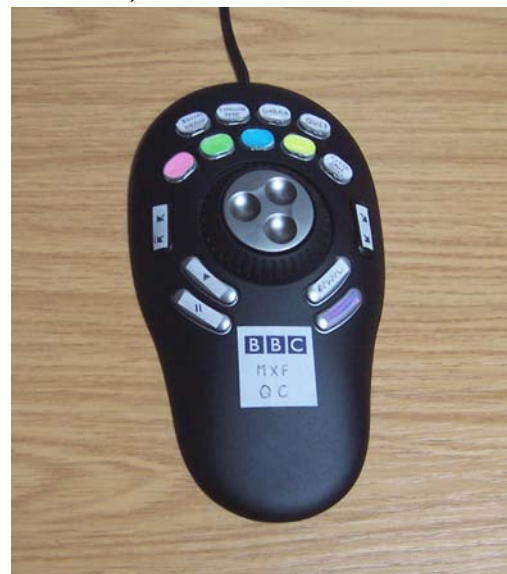
Figure 3 – USB jog-shuttle controller used by IngexPlayer
