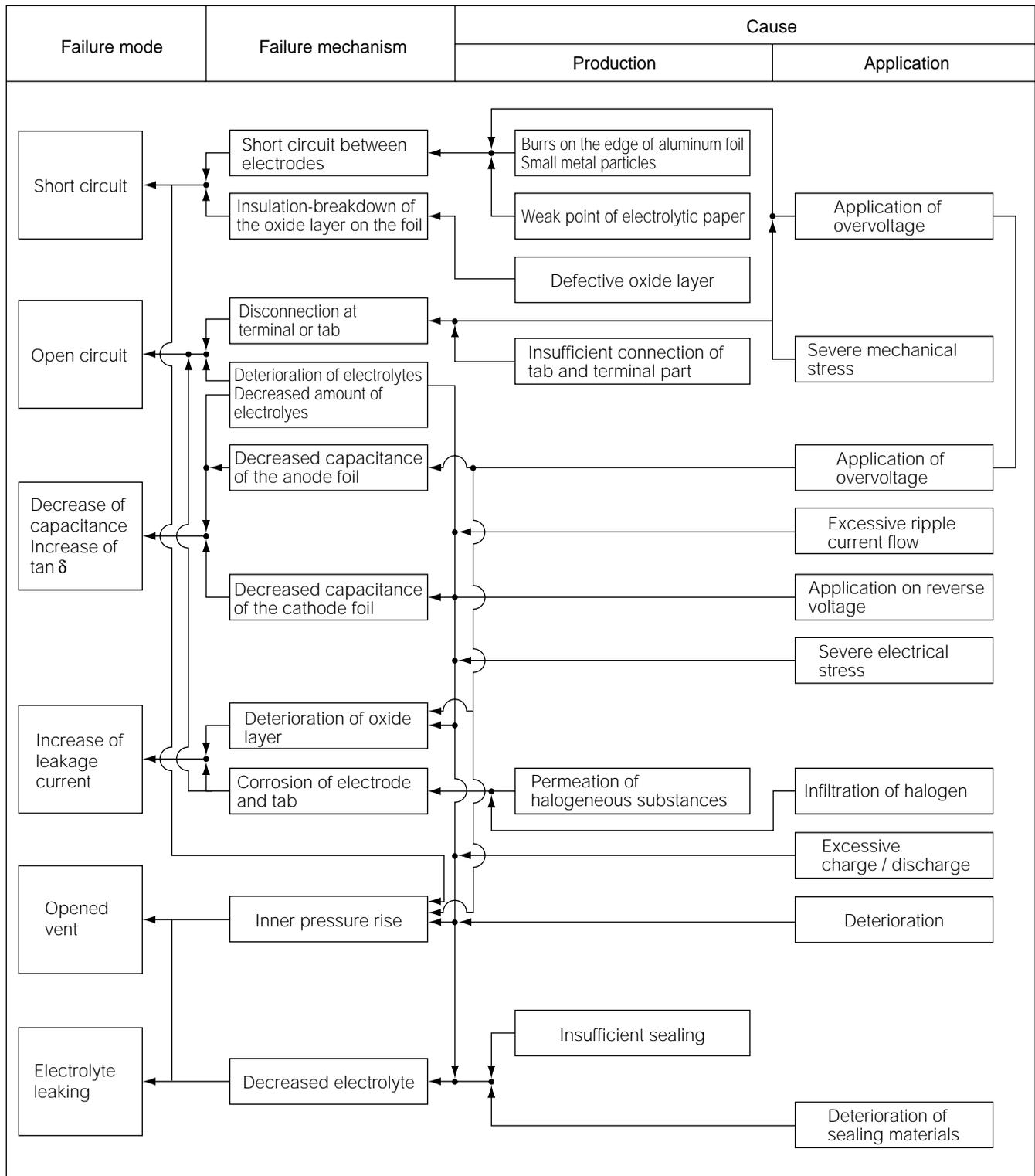
Fig. 2 - 1 Analysis of Failure Mode
