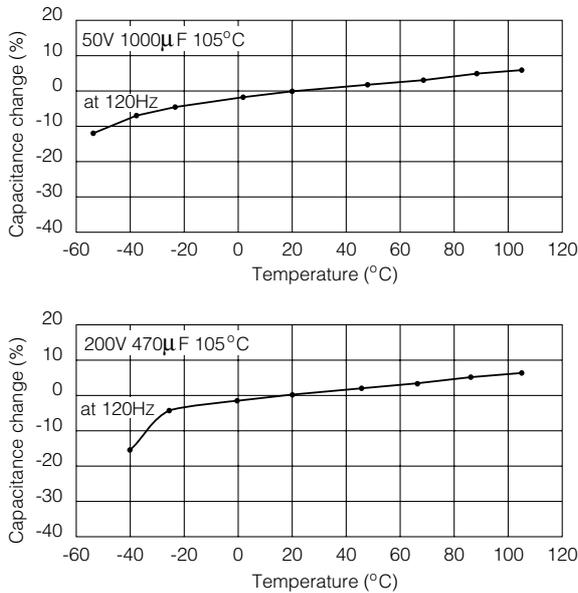
Fig. 1 - 9 Capacitance vs. Temperature Characteristics
