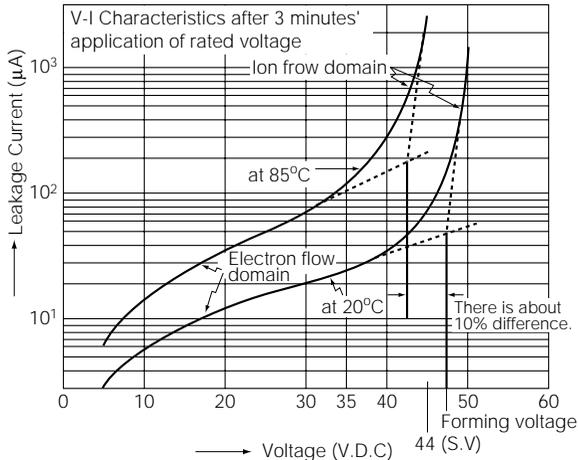
**Fig. 2-4 V-I Characteristics (ex. Rated at 35V)**
