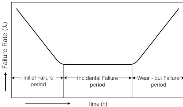
Fig. 2-11 Failure Rate Curve (Bathtub Curve)
