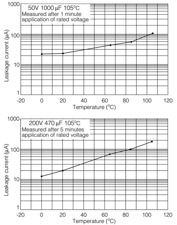
**Fig. 1 - 12 Leakage current vs. Temperature Characteristic**
