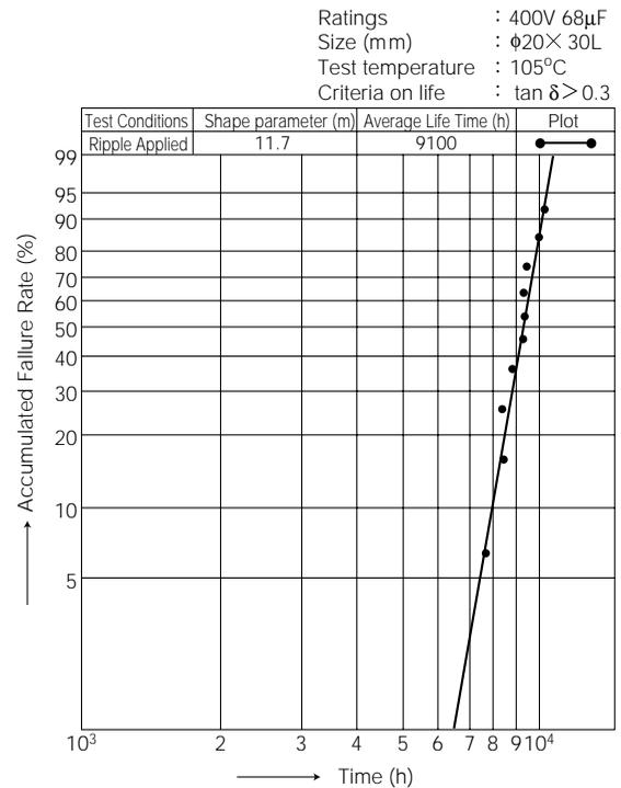
Fig. 2-12 Failure Analysis by Weibull Probability Paper
