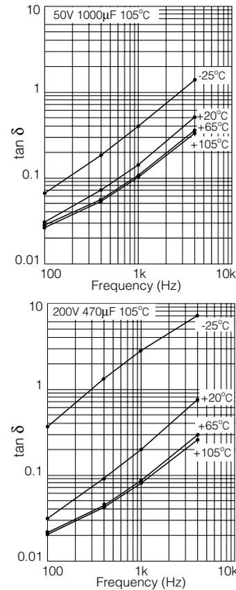
Fig. 1 - 10 Tan $\delta$  vs. Frequency Characteristics
