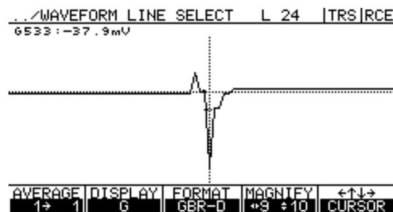
Fig. 2 Spike in green channel at red/blue transition shows an impermissible negative green level (expanded display)
