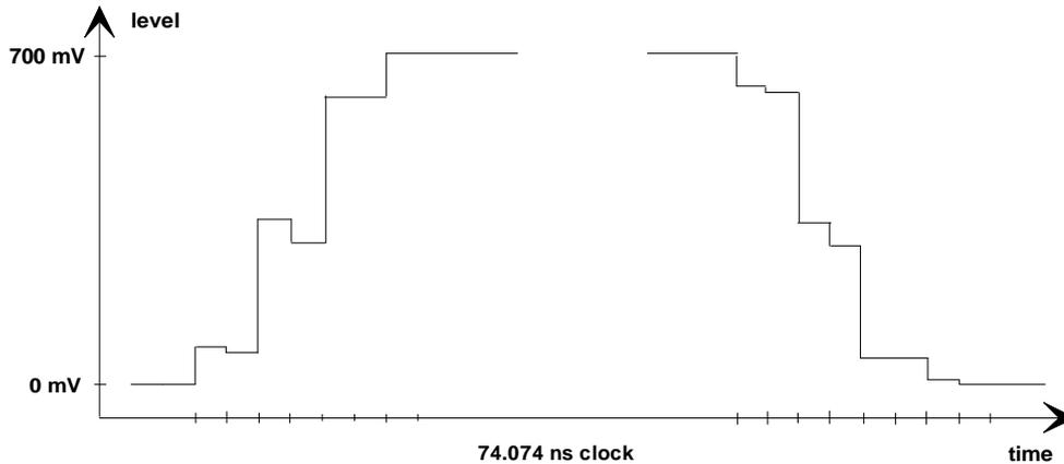
Fig. 3 The rising and falling edge in the digital R,G,B format at the digitally defined colour bar to ITU-R BT. 801
