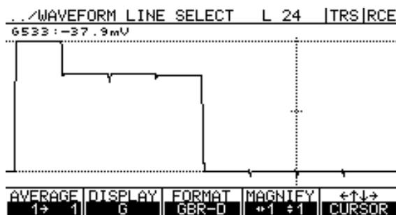
Fig. 1 Green channel of digital 100/0/75/0 colour bar on VCA display
