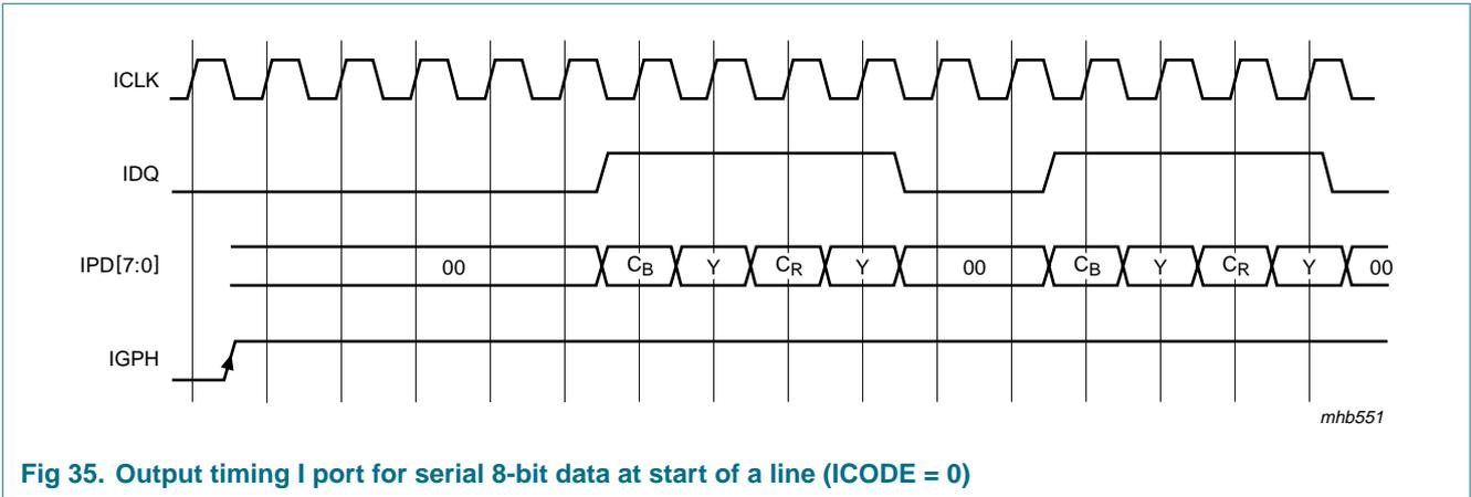
Fig 35. Output timing I port for serial 8-bit data at start of a line (ICODE = 0)
