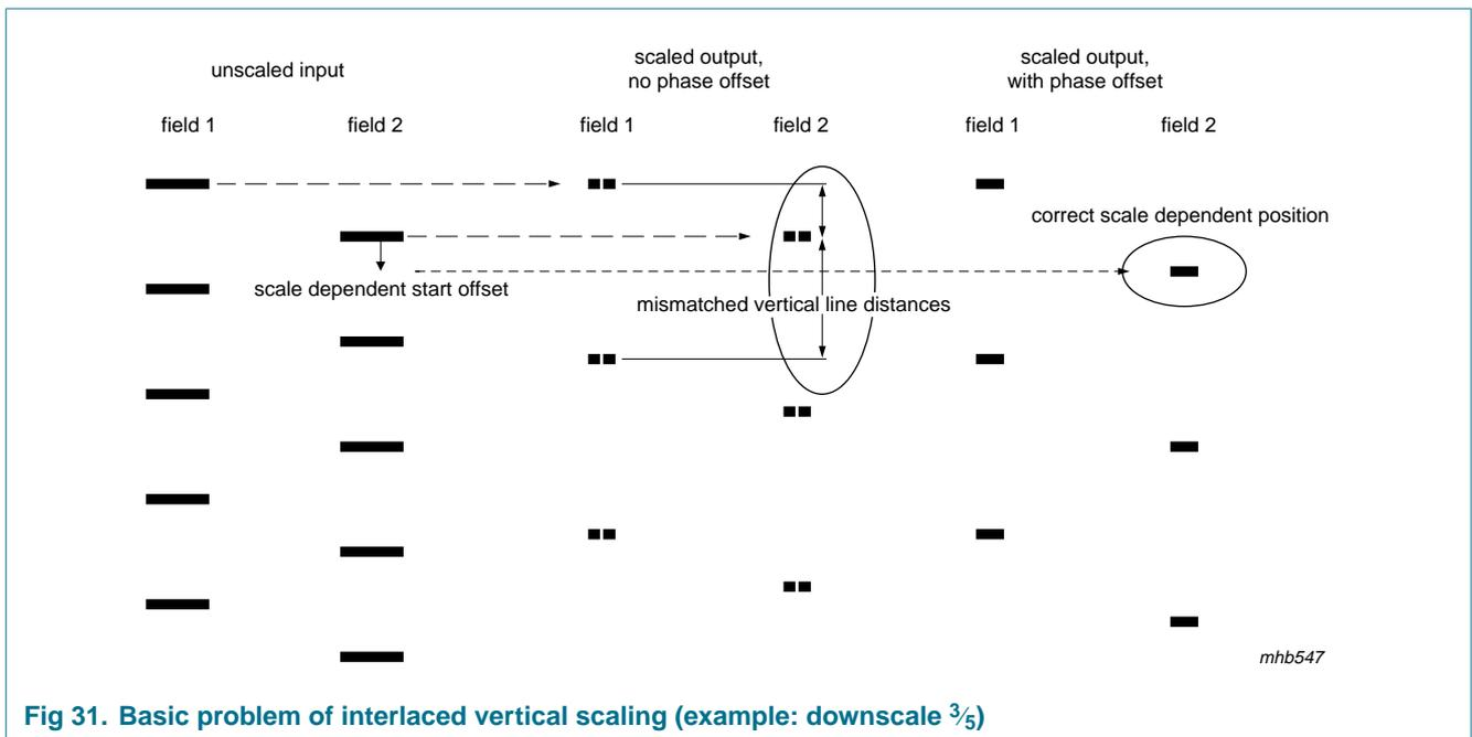
Fig 31. Basic problem of interlaced vertical scaling (example: downscale 3/5)
