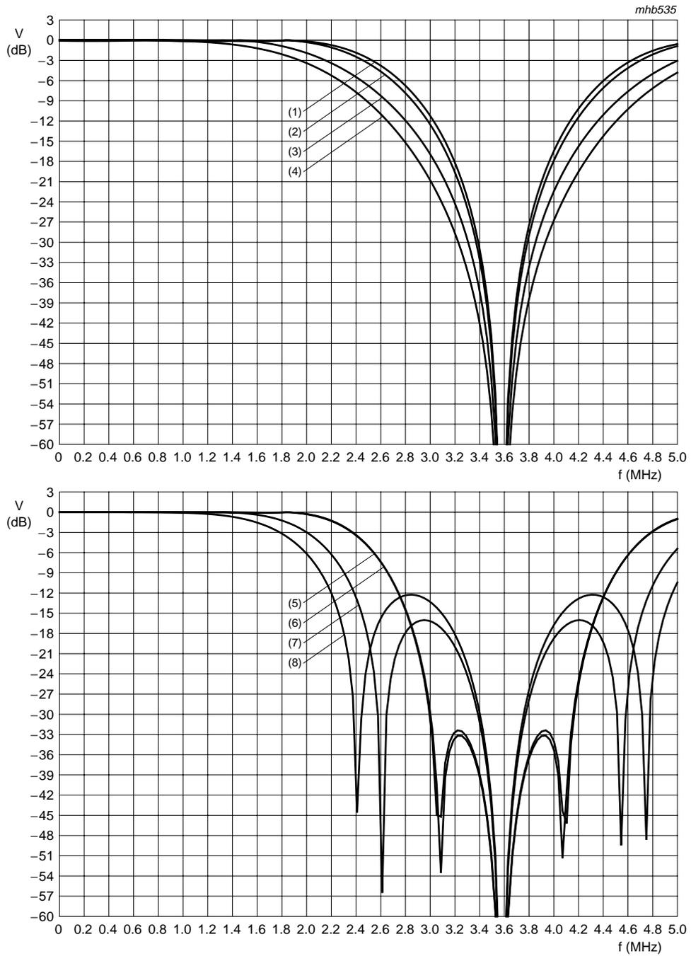
**Fig 13. Transfer characteristics of the luminance notch filter in 3.58 MHz mode (Y-comb filter disabled) at LUBW = 0**
