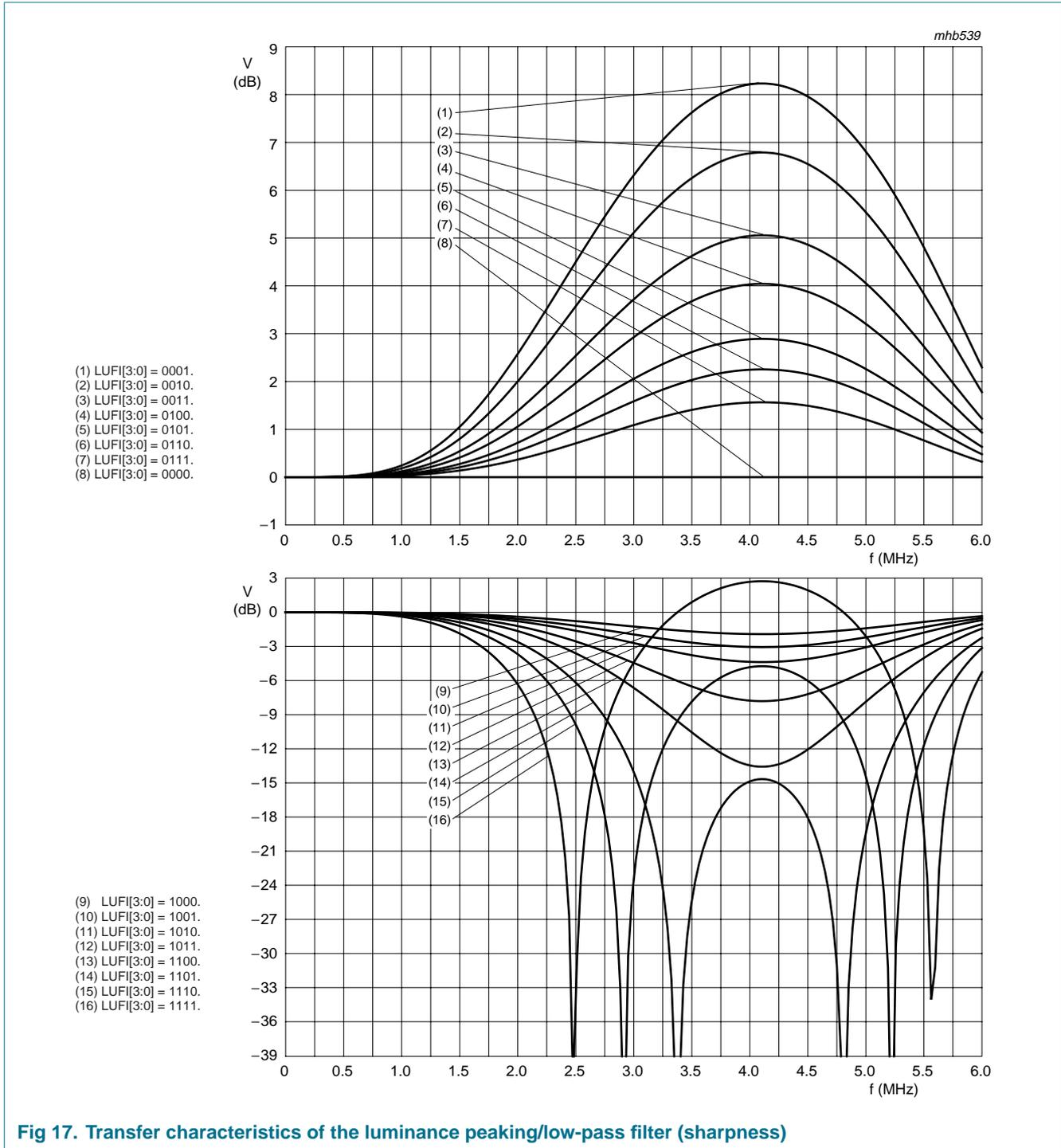
Fig 17. Transfer characteristics of the luminance peaking/low-pass filter (sharpness)
