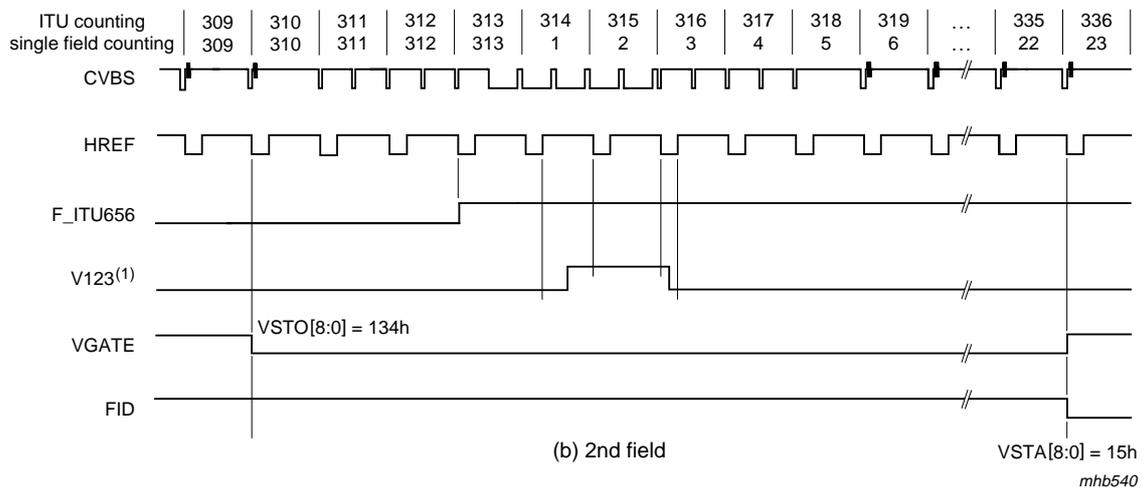
(1) The inactive going edge of the V123 signal indicates whether the field is odd or even. If HREF is active during the falling edge of V123, the field is ODD (field 1). If HREF is inactive during the falling edge of V123, the field is EVEN. The specific position of the slope is dependent on the internal processing delay and may change a few clock cycles from version to version.
