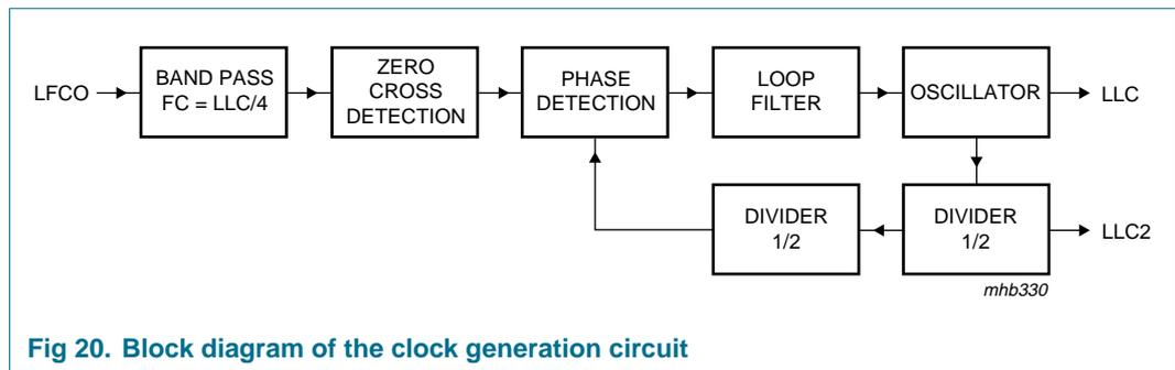
Fig 20. Block diagram of the clock generation circuit
