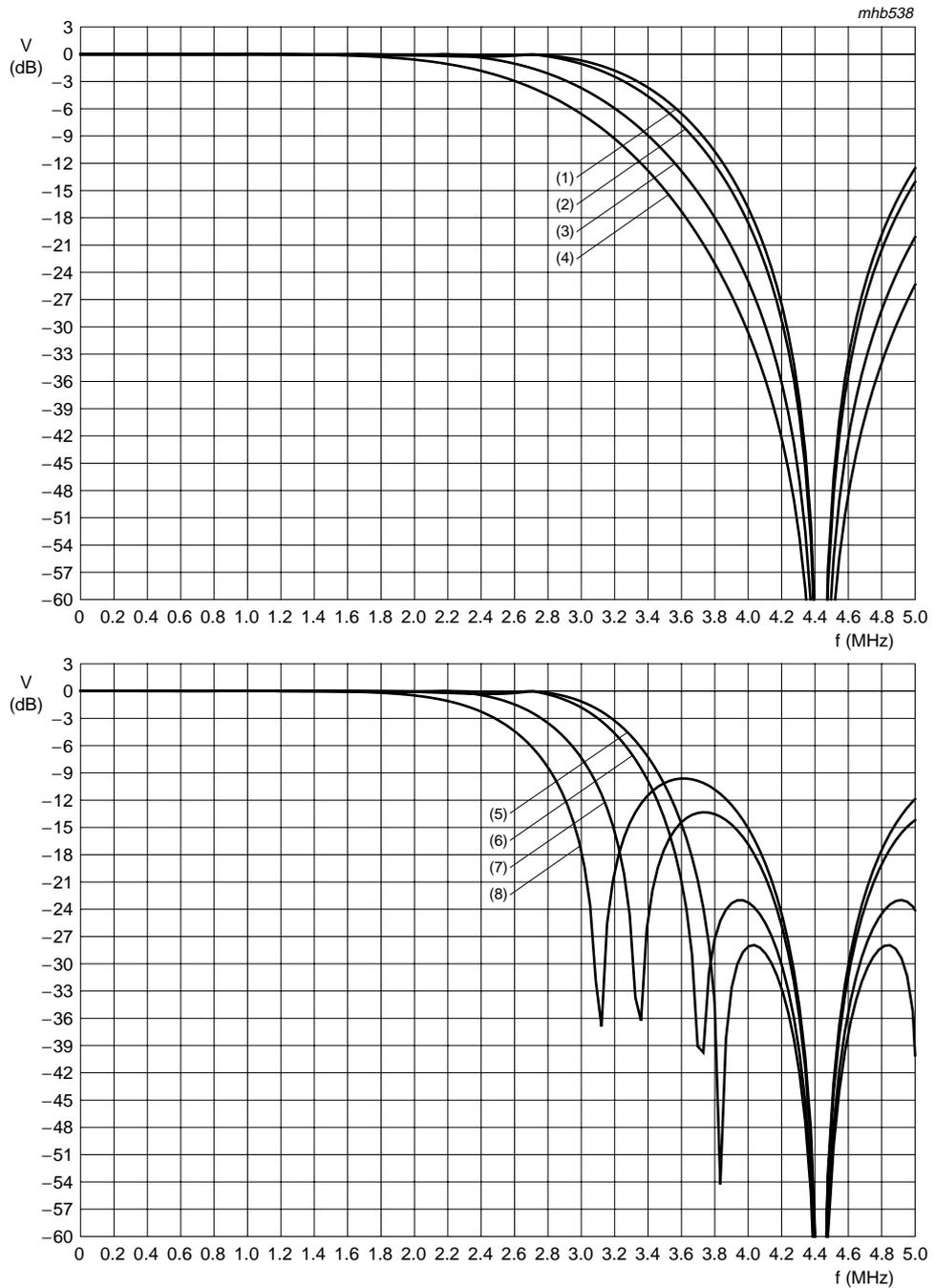
**Fig 16. Transfer characteristics of the luminance notch filter in 4.43 MHz mode (Y-comb filter disabled) at LUBW = 1**
