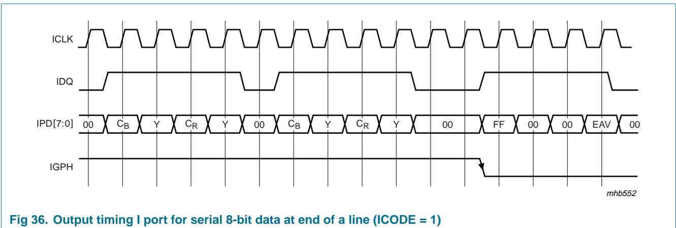
Fig 36. Output timing I port for serial 8-bit data at end of a line (ICODE = 1)
