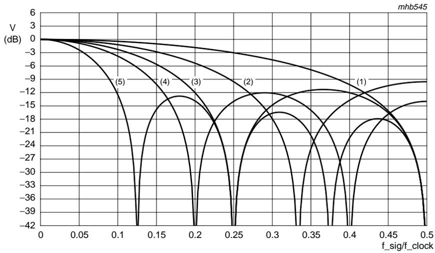
$XC2\_1 = 0$ ; Zero's at  $f = n \times \frac{1}{XACL + 1}$  with XACL = (1), (2), (3), (4) or (5)
