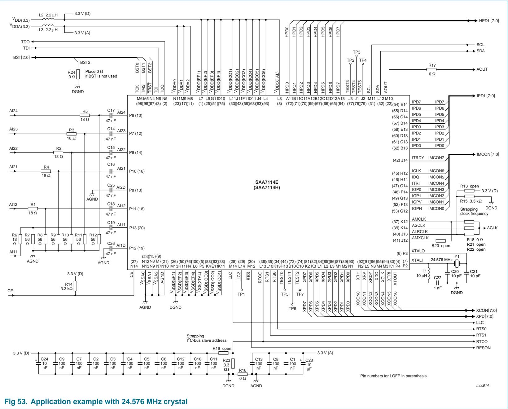
Fig 53. Application example with 24.576 MHz crystal
