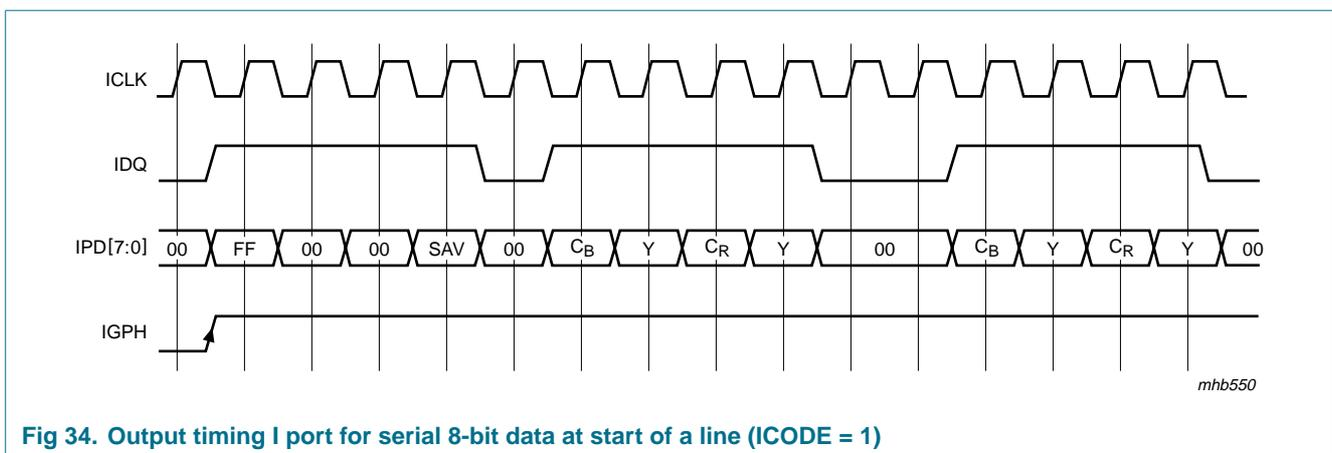
**Fig 34. Output timing I port for serial 8-bit data at start of a line (ICODE = 1)**
