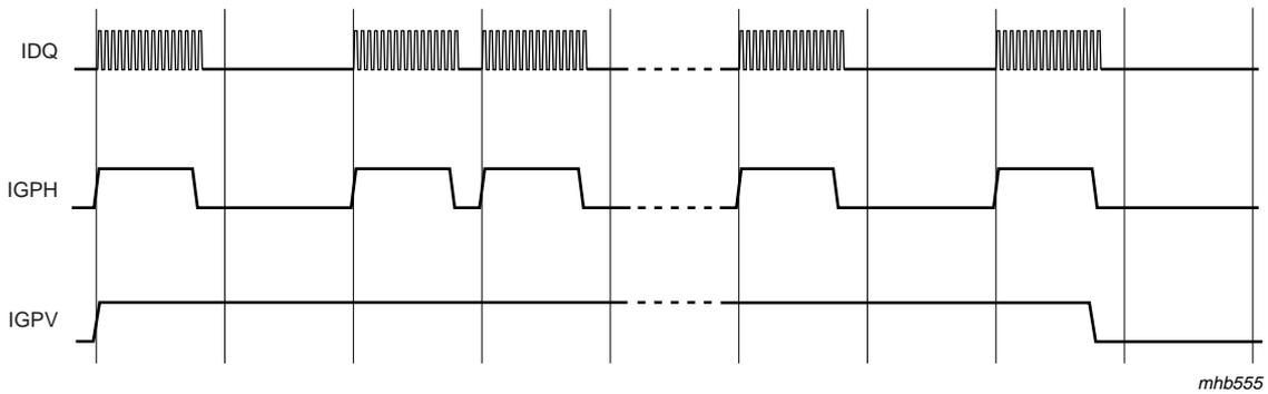
Fig 39. H gate and V gate output timing
