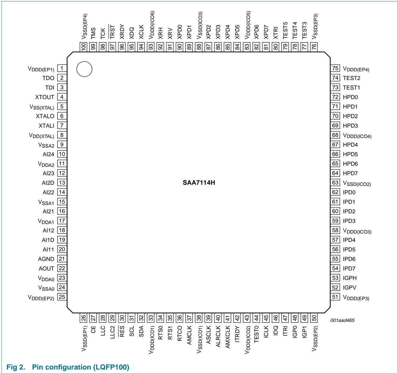
Fig 2. Pin configuration (LQFP100)
