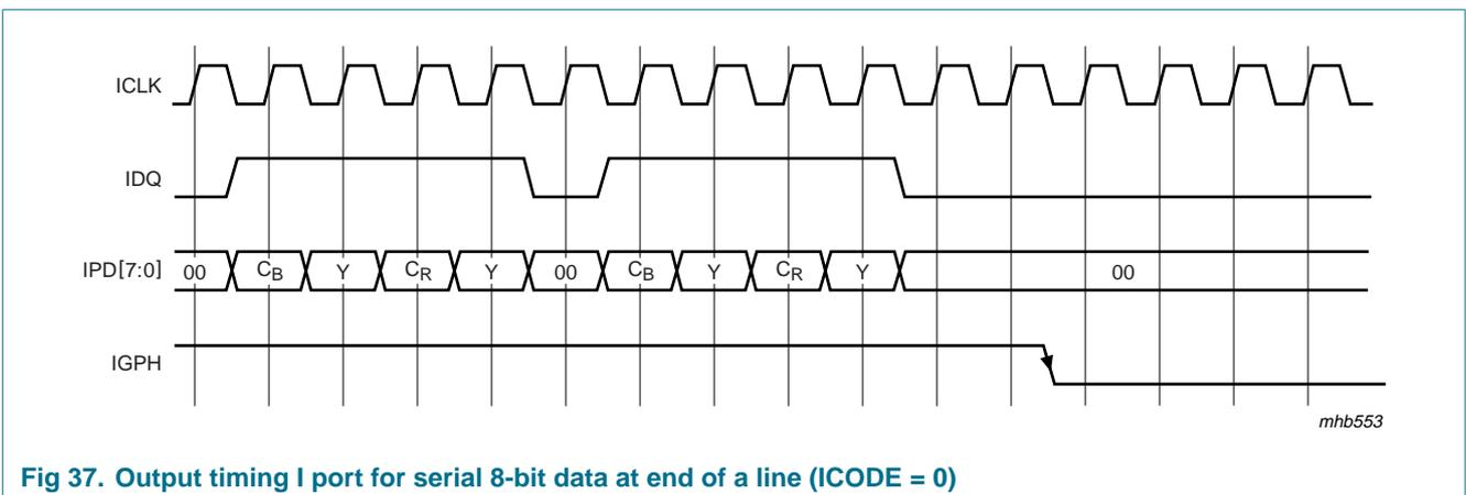
Fig 37. Output timing I port for serial 8-bit data at end of a line (ICODE = 0)
