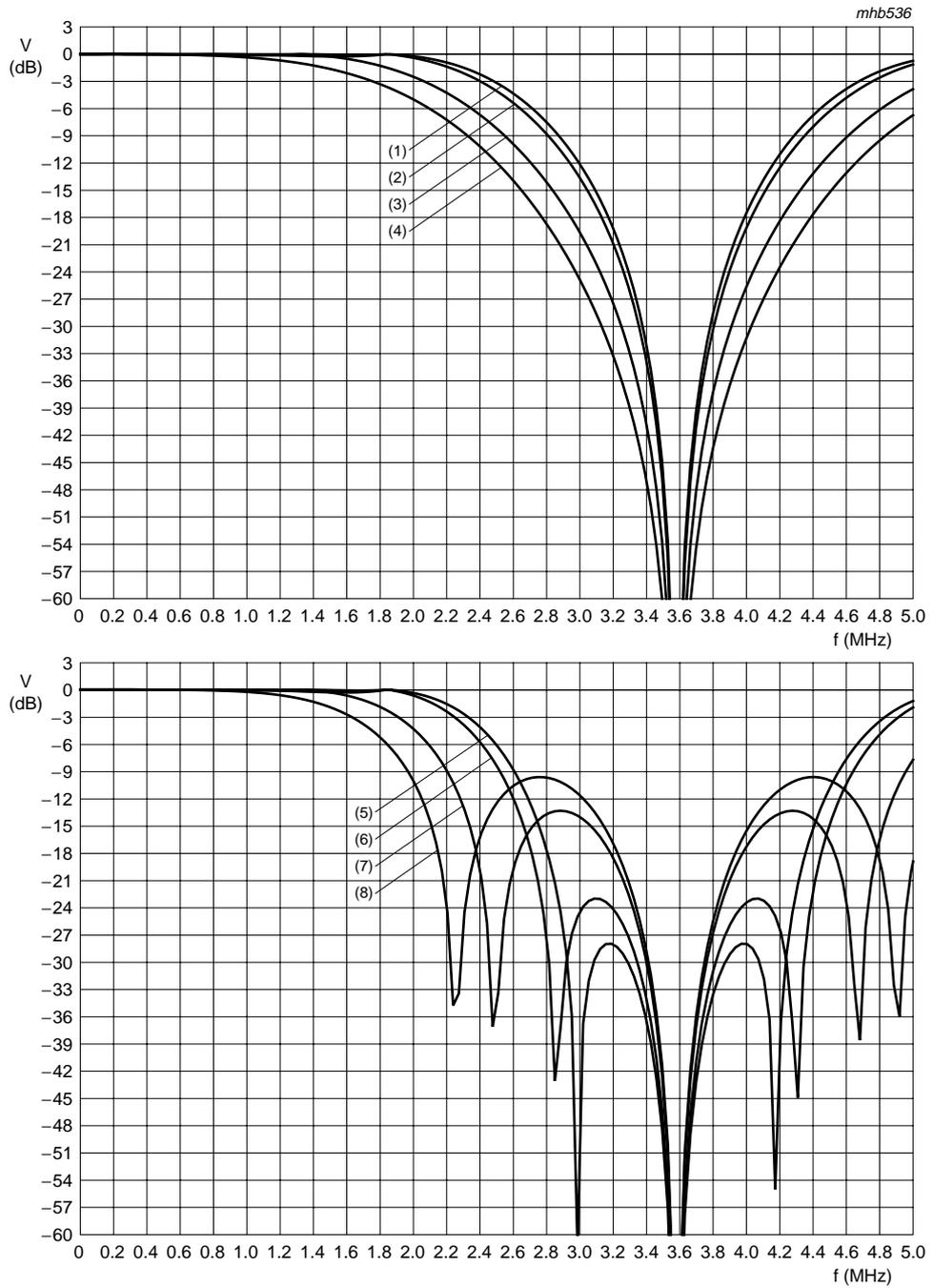
**Fig 14. Transfer characteristics of the luminance notch filter in 3.58 MHz mode (Y-comb filter disabled) at LUBW = 1**
