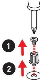
3. Tighten the base screw into the hole of the distance to the M.2 slot as the length your M.2 module.
