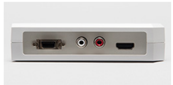
Body front. Has become from the left D input terminal, and monaural RCA pin terminal \times 2, HDMI input terminal for analog sound input
