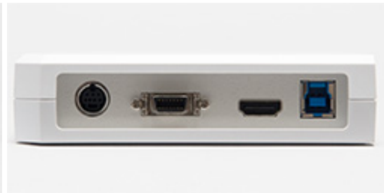
The rear body, and through the output terminal for analog AV cable, D-through output terminal, HDMI through output terminal, a USB 3.0 terminal has been prepared from the left
