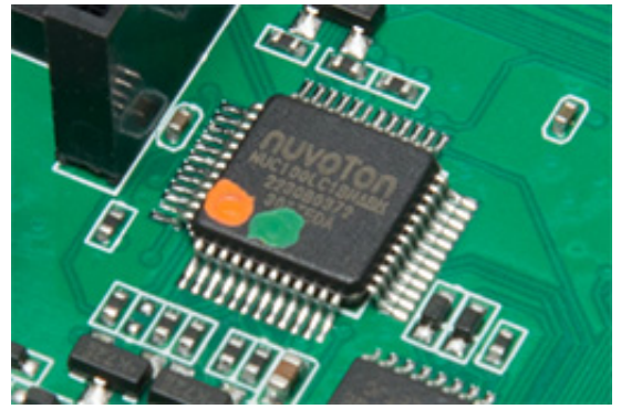
"NUC100L C18N". Although the same model number product information page of Nuvoton Technology not listed, it may have found a product that belongs to the possibly NuMicro N100 series
