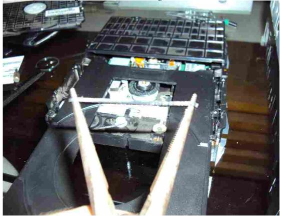
8. Upon replacement close the lid and tighten the two screws above:
