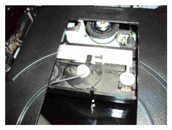
7. Remove black belt and replace with new one. Note that the former is removed and, therefore, has several grooves that causes the engine to fail:
