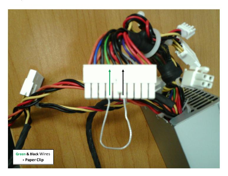
Once the paper clip has been attached to the green and black wires, this will enable the power supply to turn on while it is disconnected from the mother board something not possible, otherwise. After this is done, turn off the power switch, if one is present, and connect the power cord to the PSU as shown below:
