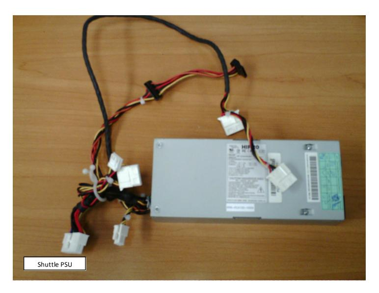
When a PSU fan goes bad, it is not able to cool down the power supply hence the device will heat up. The excess heat generated by the PSU will add to the overall temperature of the system unit. If this failure is not corrected, the PSU will become damage. A damaged PSU can, potentially, damage the components as well as the motherboard, itself.
