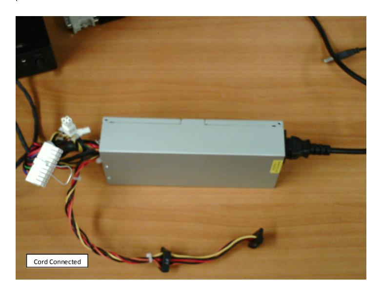
If the PSU does not have a switch, then as soon as you connect the power cord, power should flow through the PSU and you can then observe the fan on that power supply to see if it turns as shown in the image that follows:
