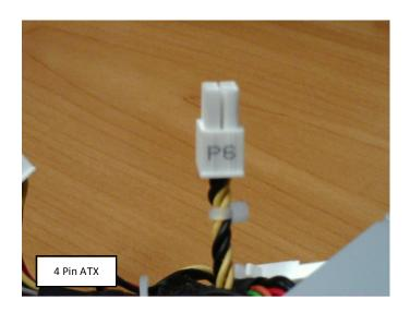
These connectors are needed by your motherboard in order to function properly. As mentioned above, they supply the proper voltages and currents that the various components attached to the motherboard need in order to work properly. These components include, the motherboard itself, the CPU, the memory modules, the hard drive and the optical drive as well as any video cards that your system my use.
