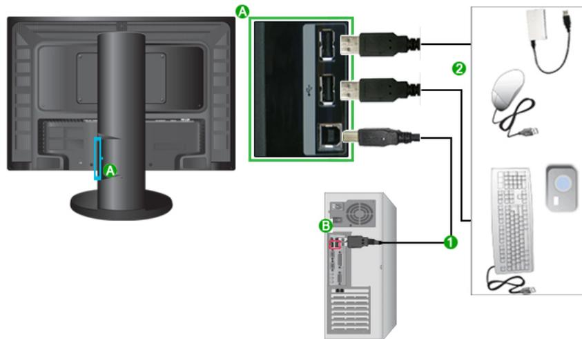
1. Connect the
