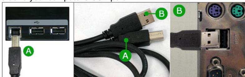
2. Connect the *DOWN* port of the USB monitor and a USB device with the USB cable.
