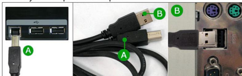
2. Connect the
