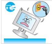
▶ When you drop the product or the case is broken, turn the power off and disconnect the power cord. Contact a Service Center.
