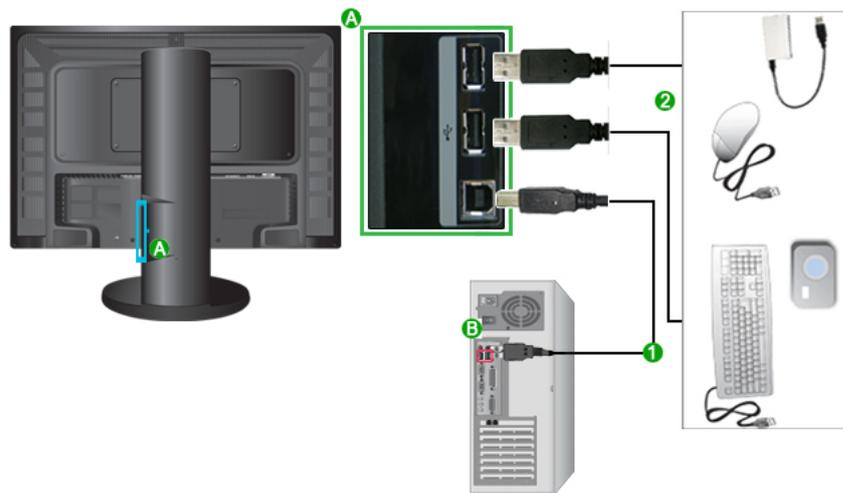
1. Connect the *UP* port of the monitor and the USB port of the computer with the USB cable.
