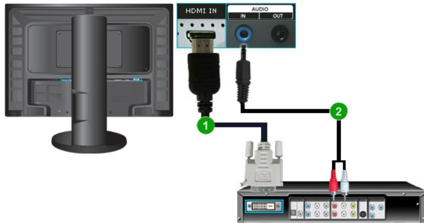
1. Connect the DVI output terminal of a digital output device to the *HDMI IN* terminal of the monitor using a DVI to HDMI cable.
