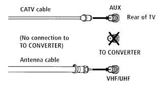
Select CABLE or antenna (ANT) mode by pressing ANT on the remote control.
