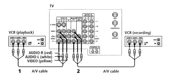
To perform tape editing, set the TV to the video input intended for playback by pressing the TV/VIDEO button on the remote control.
