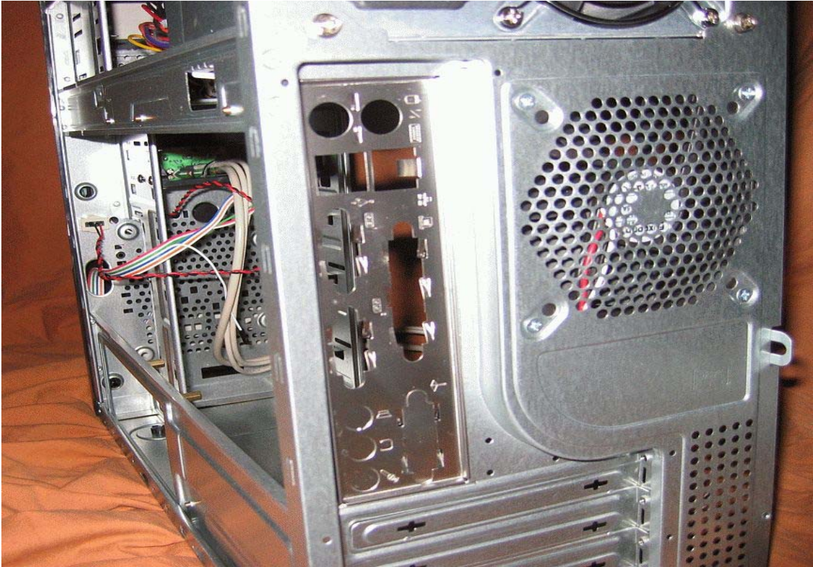
Photo 14. The generic motherboard connector panel. Just pop it inwards and use the one included with the motherboard.
