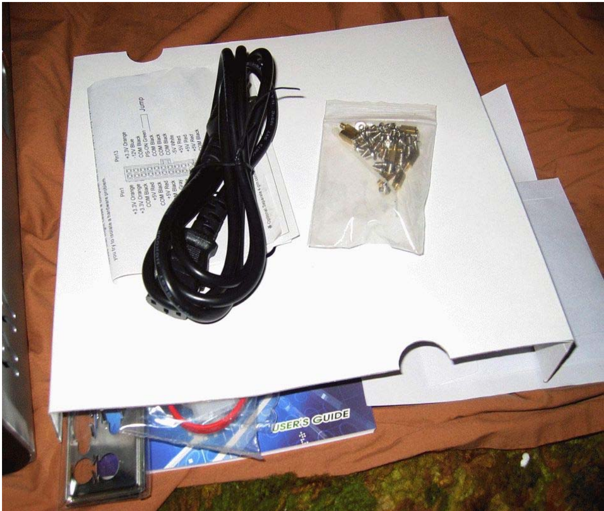
Photo 9. The parts included with the case. A line cord, a package of screws and an assembly instruction paper. Don't lose this. It has the front panel wiring diagram on it.
