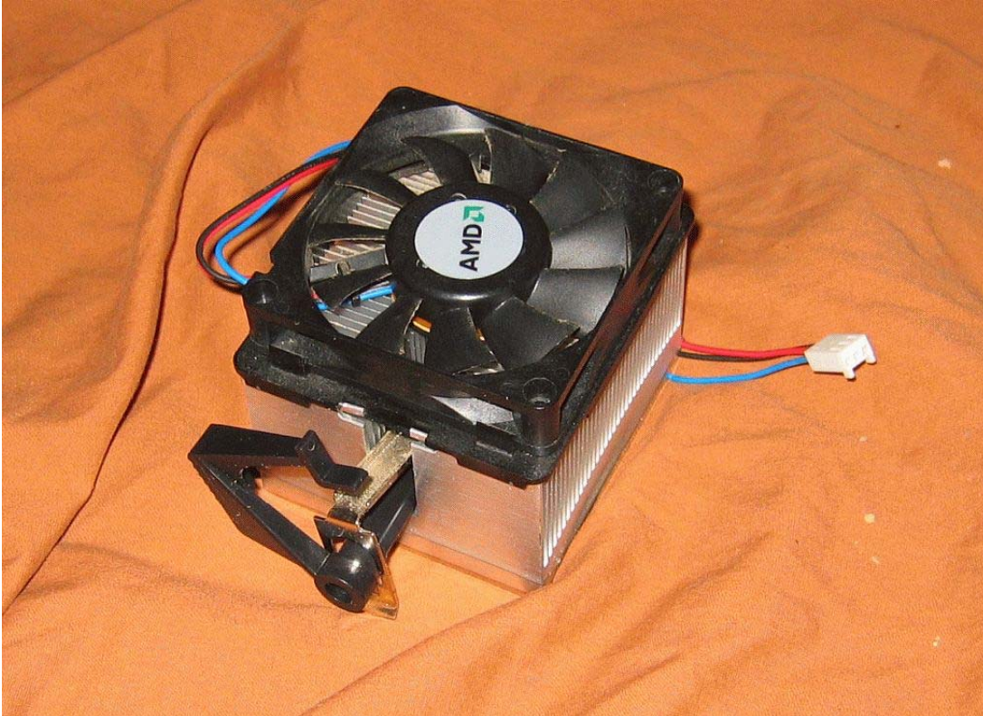
Photo 5. The CPU cooler. This is a Standard AMD model included with the CPU. This one is used. The hold down latch is slid out to one side. It's fairly quiet and sufficient for most uses.
