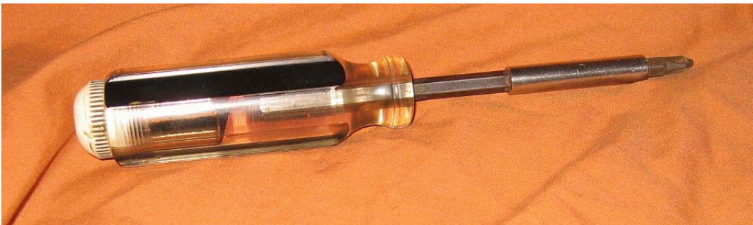
Photo 6. The only tool you need. I like the replaceable tip Phillips #2. You definitely want a magnetic tip so you don't drop screws down into the case.
