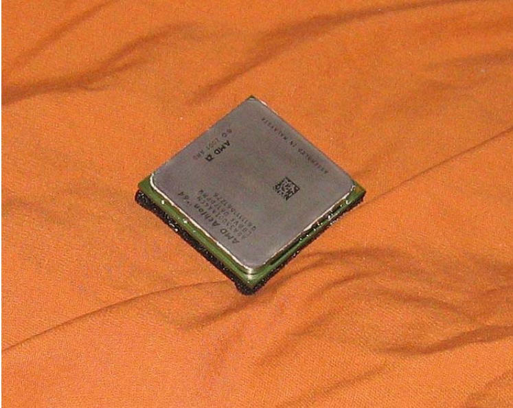
Photo 7. The AMD AM2 Athlon 3800+ CPU. It's sitting on an antistatic pad. This one is used. I cleaned off the old thermal compound with a fingernail and 99% isopropyl alcohol on a dampened Q-tip. Same for the cooler. Be careful not to scratch either surface. Don't get any fingerprints or oils on the CPU heat spreader or CPU cooler surface. Clean them off if you do.
