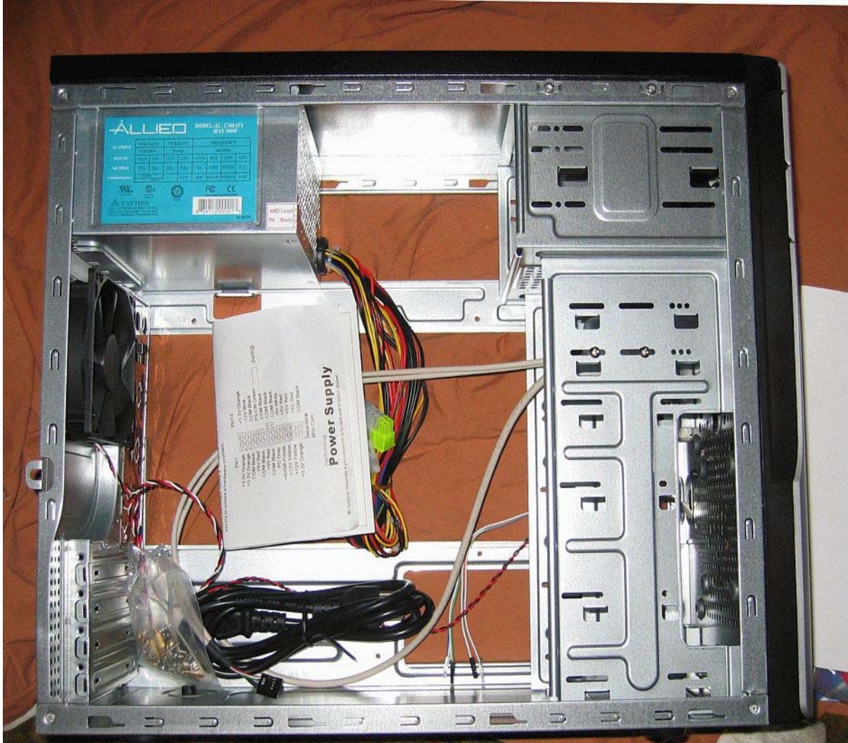
Photo 8. The case with the four rear screws and the two side panels removed. It's a good quality case with an included power supply that is big enough for this type of computer. There are no sharp edges or poor fits that you may see with some cheaper cases. It has a rear exhaust fan included.
