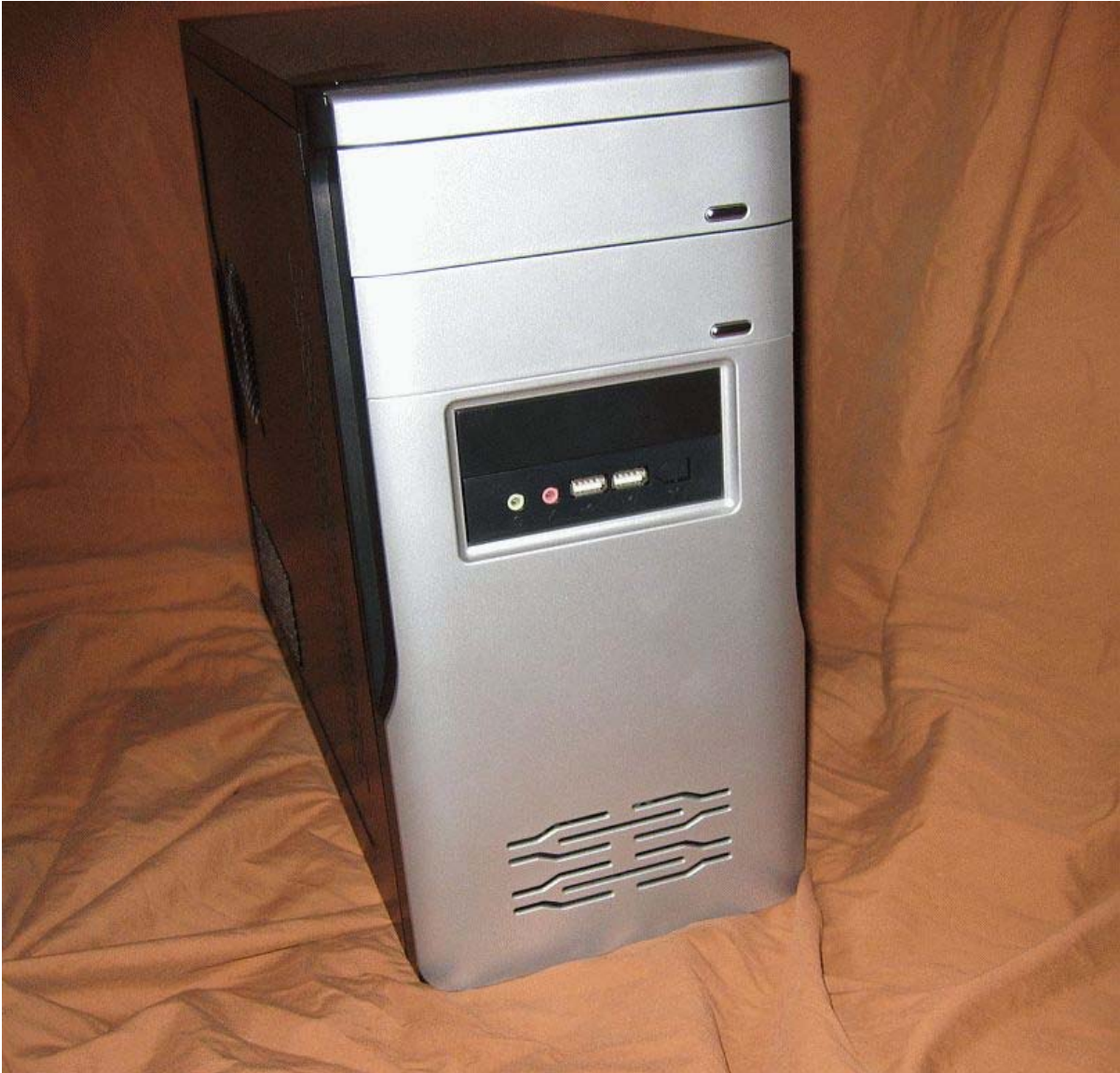
Photo 2. The Micro-ATX case. I somewhat dislike the doors in front of the optical drive as you need to push on the DVD tray to close it instead of using the now hidden open/close button. I probably wouldn't use this type of case again. It is well built for my purpose, but I failed to note the type of 'doors' when I ordered it. You could also use a mini-tower case, which are only a few inches bigger all around. If you use a full size ATX motherboard, you will need the mini-tower size. They also have a little more room to work in, and have generally better cooling options.
