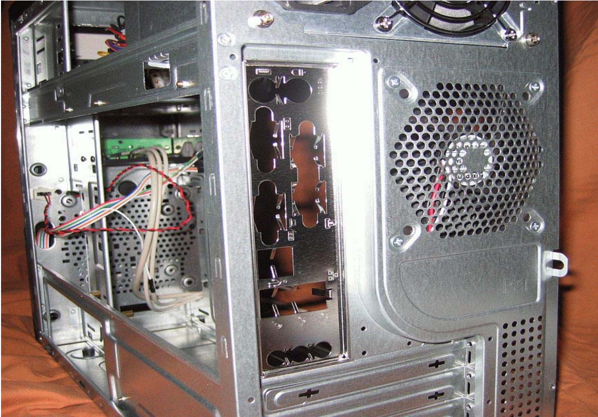
Photo 15. The proper motherboard connector panel for the ECS motherboard. Try not to bend it when inserting and make sure it is seated evenly all around in the opening.
