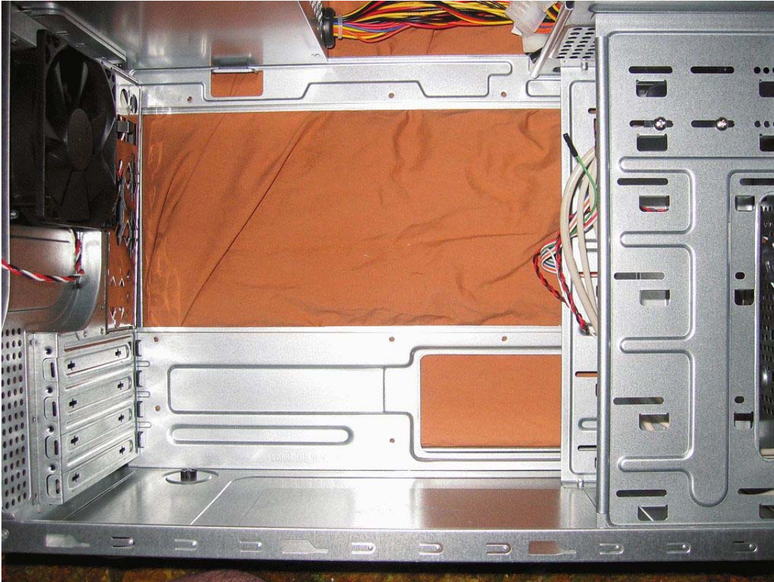
Photo 10. The case with all the wiring pulled out of the way, laid on its right side. This is the best way to work on it at this stage.
