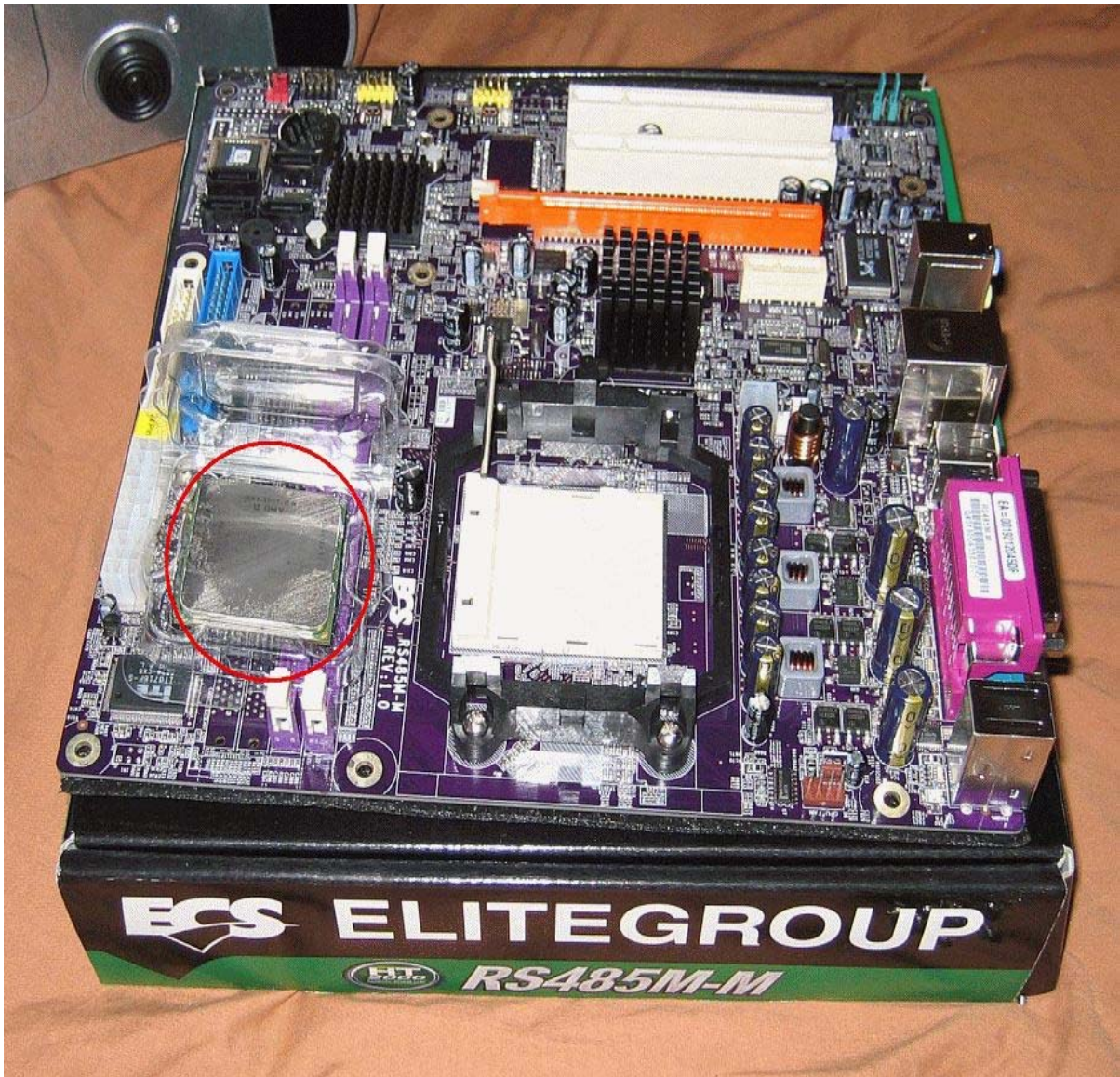
Photo 18. The motherboard, along with the CPU. Notice the retention arm is raised to a 90 degree angle, ready to accept the CPU.
