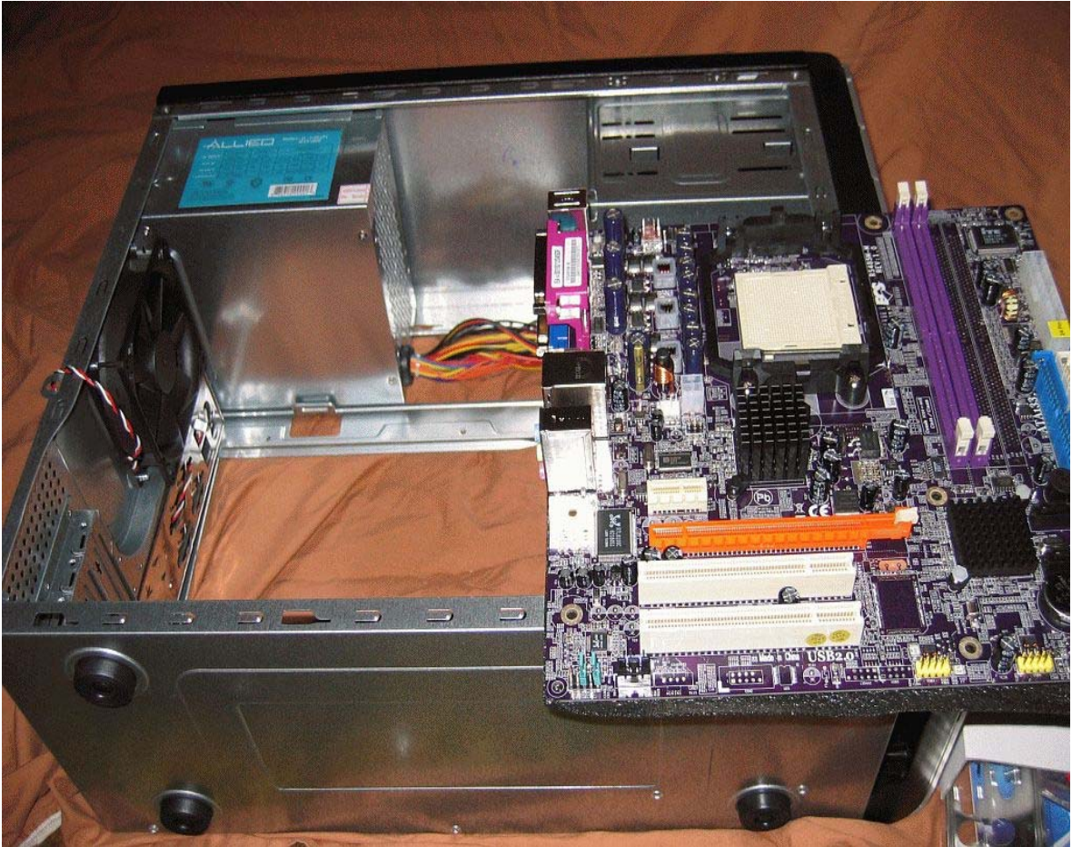
Photo 11. Checking the motherboard for fit and seeing where the mounting holes line up with the case.
