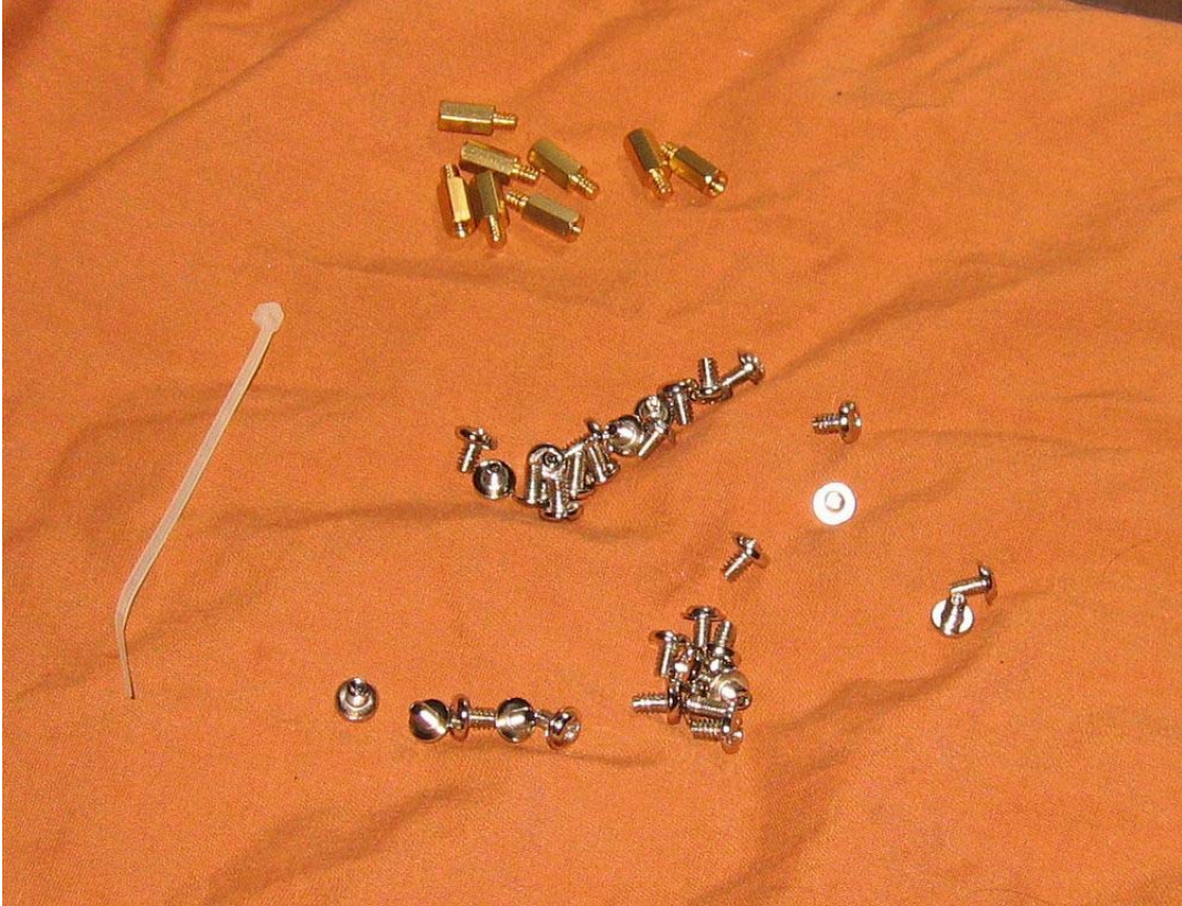
Photo 12. The contents of the case screw package. The motherboard standoff mounts are to the top, below are the optical drive mounting screws and at the bottom, the motherboard mounting screws and the screws for the hard drive mounts. There is also a token zip tie. Get about 20 of these, in 4 inch length as you will need them later.
