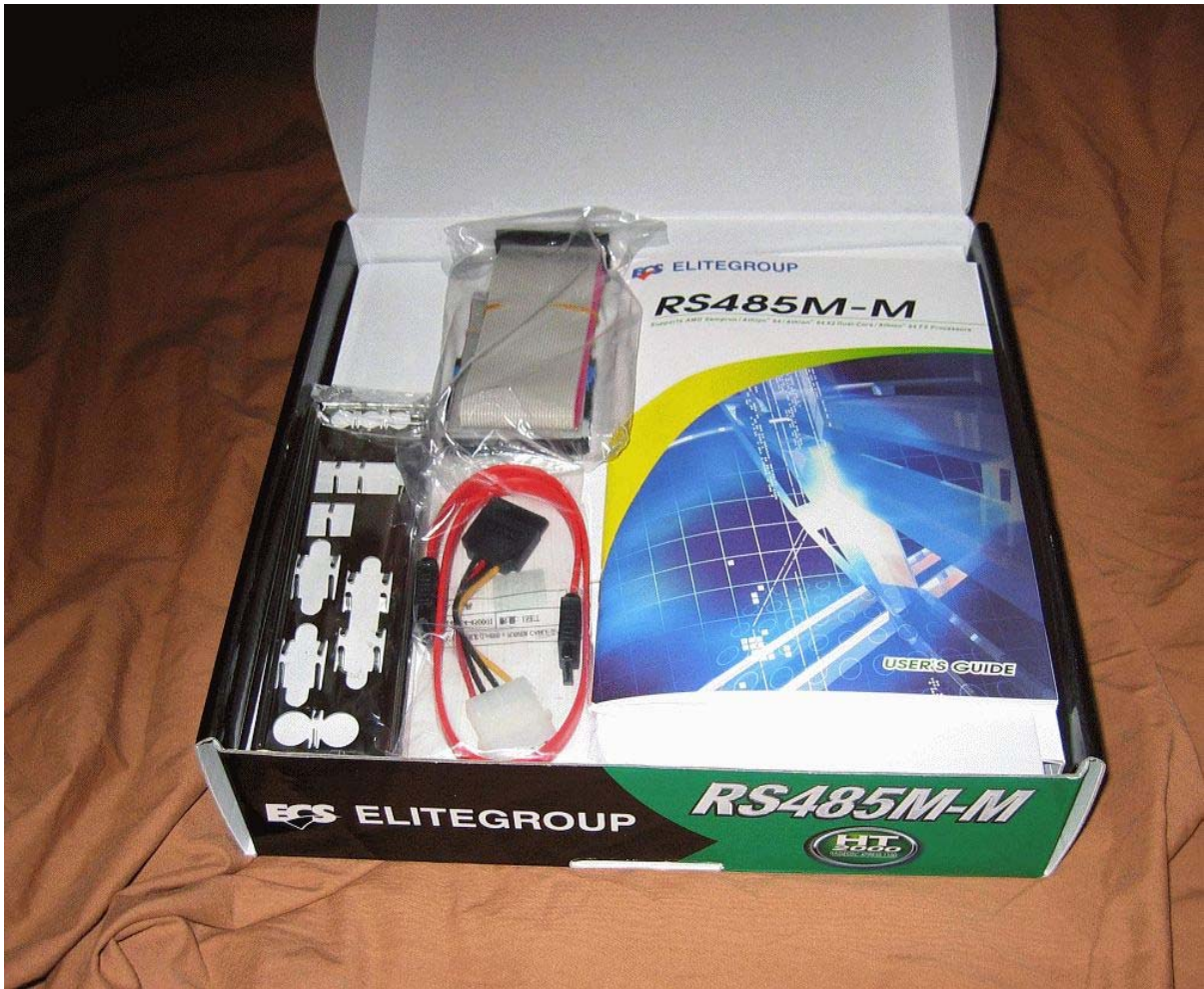
Photo 3. Parts included with the motherboard. There are a couple of ATA cables, a SATA cable and the rear connector panel, along with a motherboard manual and a CD disc of motherboard drivers. The motherboard is underneath, wrapped in an anti-static bag.
