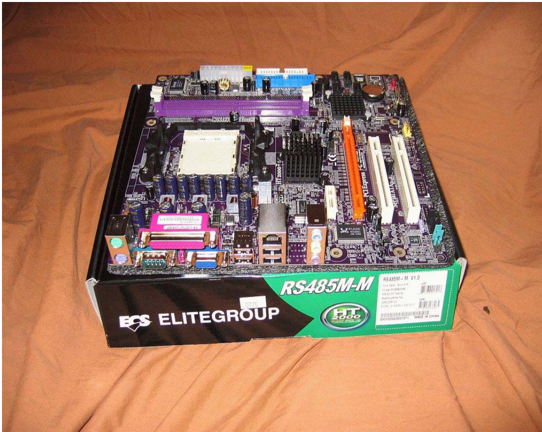
Photo 4. The motherboard. It is sitting on the anti-static pad it came with. Keep this pad on the MB until you are ready to install it.
