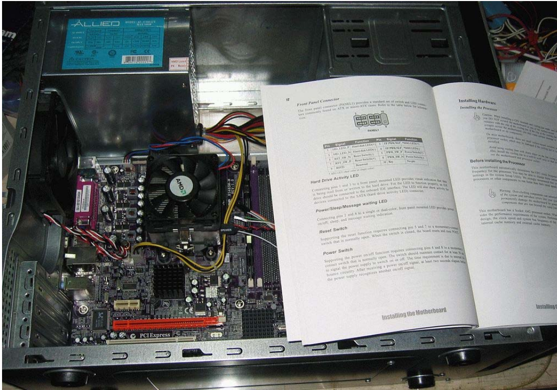
Photo 31. Front panel connections. This part can be difficult, but there is no easy way to do it until the motherboard is installed. I usually open the motherboard manual, and have the case wiring paper handy for this. It's almost always cramped where the panel connectors are, usually near the bottom right side of the motherboard. It helps sometimes to turn the case around to be able to see in there better. Lots of light helps also. Fortunately, most front panel cables are labeled. And the good news is even if you get every one of them wrong, it won't cause any damage to the motherboard or the case. Pay attention mostly to the + and - markings for the LED indicators or they won't work. The switches and speaker connections won't be a problem for polarity.
