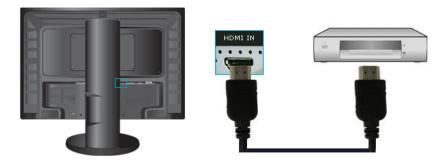
1. Input devices such as digital DVD are connected to the *HDMI IN* terminal of the monitor using the HDMI cable. When all the connections are completed, connect the power cords for the monitor and DVD (or the device connected to the digital output terminal).
