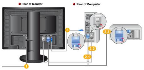
Connect the power cord for your monitor to the POWER port on the back of the monitor.
