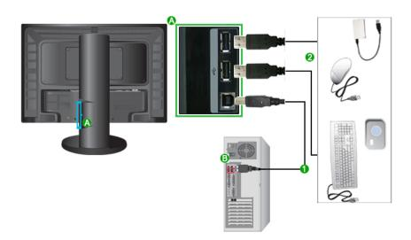
Connect the UP port of the monitor and the USB port of the computer with the USB cable.
