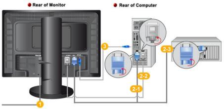
Connect the power cord for your monitor to the POWER IN port on the back of the monitor.
